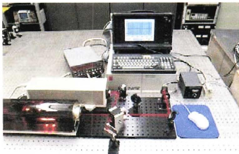
**Figure 3. Length calibration.** The photo shows an iodine stabilized HeNe laser (in the foreground), which is used as a length standard to calibrate the wavelength of a second laser (behind the iodine stabilized laser). The calibrated second laser is then used for ultra-high precision measurements in both laboratory and industrial settings. The laser in the photograph was built by Jack Stone of NIST.
