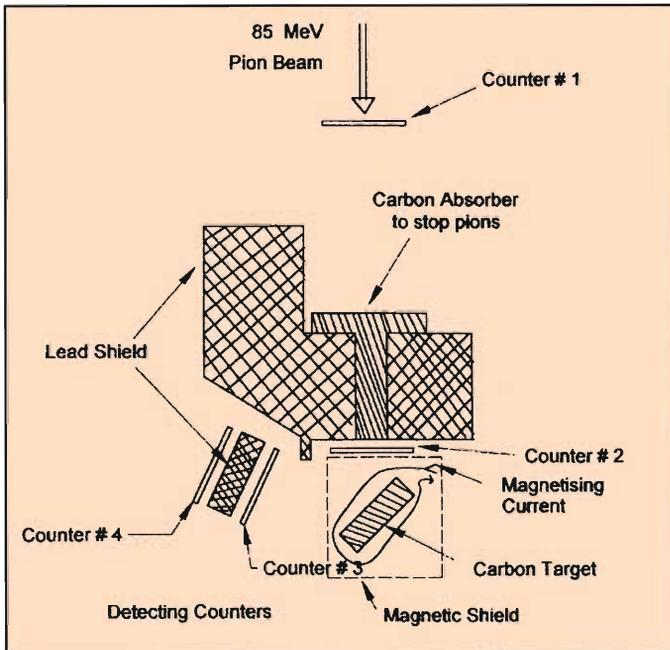
*Figure 3. Sketch of the experimental arrangement of Garwin, Lederman and Weinrich. (Reproduced from Physical Review Letters, Vol. 105, pp.1415-1417, 1957 with permission from American Physical Society).*
