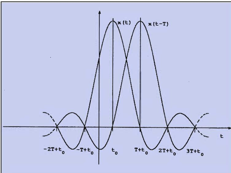
**Figure 4. Condition for avoidance of ISI – the pulses equal zero at all sampling times except their own.**
