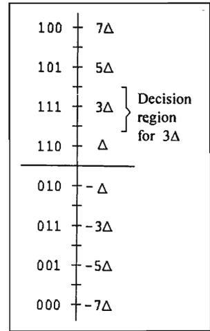
**Figure 3. Pulse amplitude levels chosen from 8-level alphabet.**
