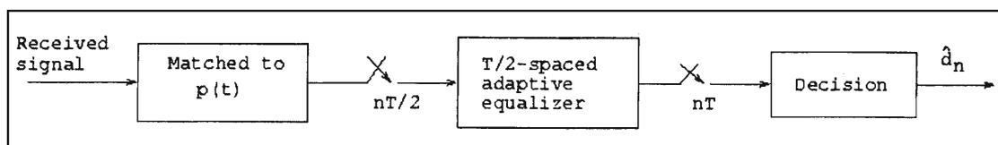
**Figure 7. A receiver structure when the channel is non-ideal and unknown (a desired structure in practice).**
