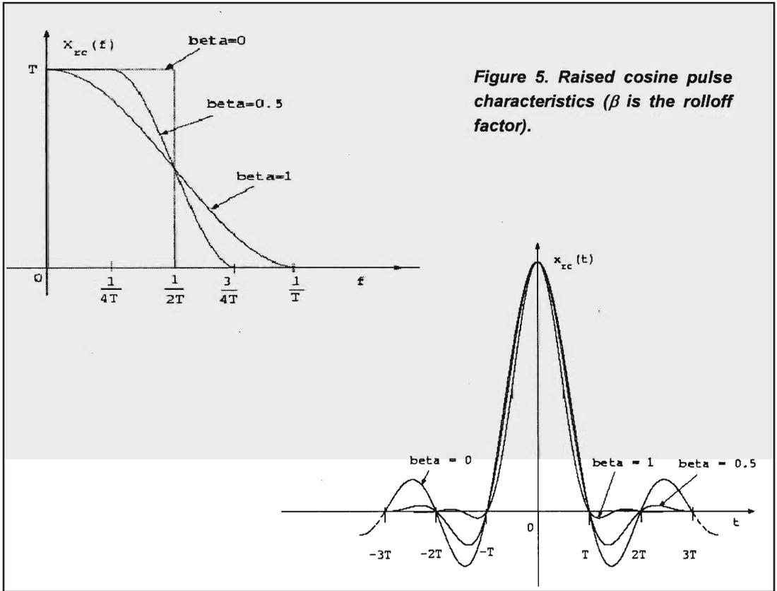
Figure 5. Raised cosine pulse characteristics ( $\beta$  is the rolloff factor).
