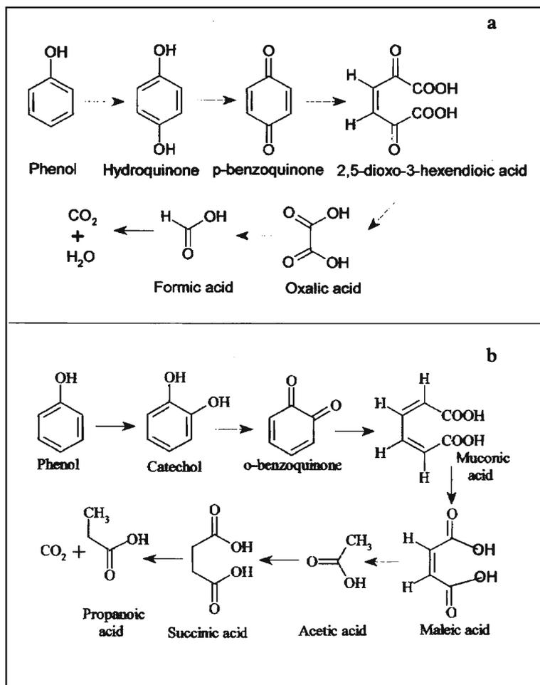
oxidation of phenol in wastewater. Degradation pathway is likely to change with the change in the intensity of ultrasound, concentration of the contaminant in water, etc. An unanticipated advantage is that sonication also kills some microorganisms and hence disinfects water.
