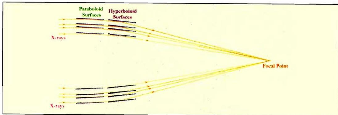
**Figure 2a.** A schematic of the grazing incidence of X-ray telescope, showing how the X-rays ricochet off the mirrors.
