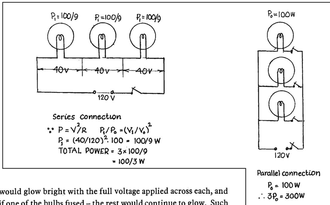
**Figure 3. Series and parallel connection of bulbs.**
