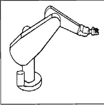
**Figure 2. Manipulator arm with three limbs.**
