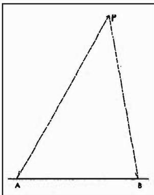
**Figure 1.** The method of triangulation. Observers at A and B will measure the angles PAB and PBA. The triangle can be reconstructed to get the altitude of an object at P.
