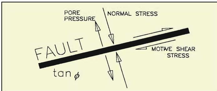
*Figure 3. Quantities required to specify condition for slip on a fault. All refer to the same point in the fault.*
