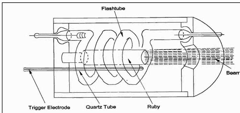
**Figure 2.** The schematic of apparatus used by Maiman and co-workers for the ruby laser.
