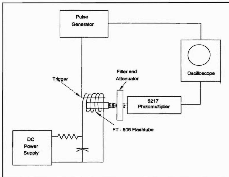
Figure 3. Schematic diagram of the electronics for ruby laser.
