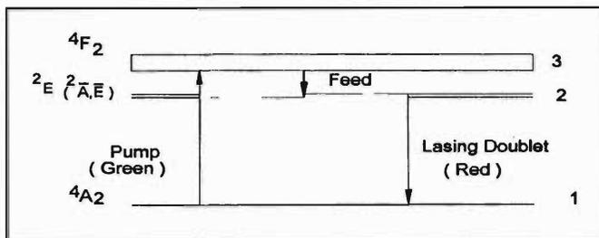
Figure 1. The energy levels of ruby used for the laser action.
