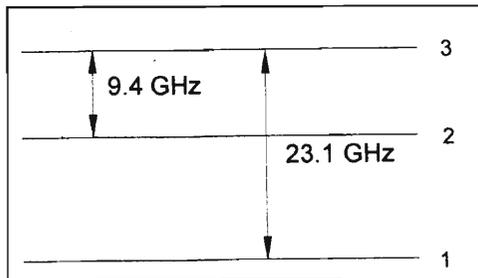
Figure 3. The three level maser system using the excited levels of ruby.
