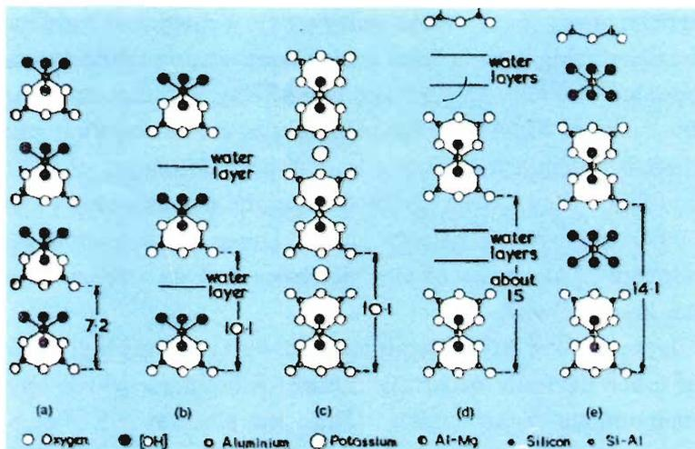
Figure 3. Schematic representation of layers of clays: a) kaolinite, b) hydrated halloysite, c) muscovite, d) hydrated montmorillonite, e) chlorite.
