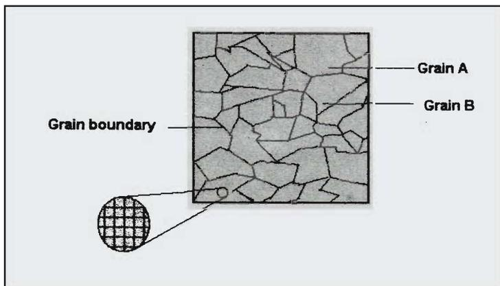
*Figure 1. Schematic representation of grains and grain boundaries in a ceramic material. Each grain is made up of many single crystals.*
