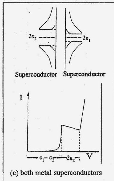
***I - V characteristics for the tunneling current between (a) two metals (b) superconductor-metal and (c) two superconductors separated by a thin layer of insulator.***
