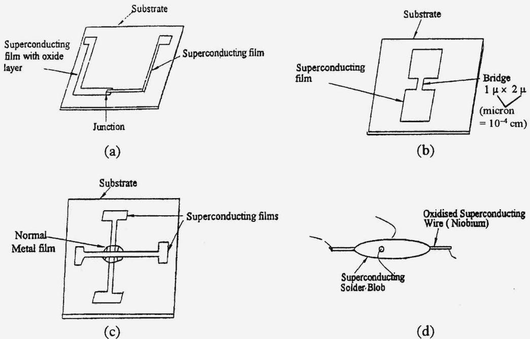
*Different types of Josephson tunnel junctions (a) Josephson tunnel junction; (b) Dayem bridge; (c) S-N-S junction; (d) SLUG.*
