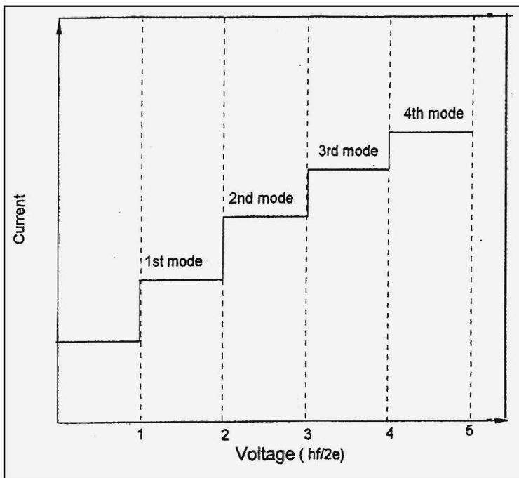
Figure 4. The effect of applying microwave to a Josephson junction. The steps in the I-V curve occur at multiples of  $(hf/2e)$ , verifying the ac Josephson effect.
