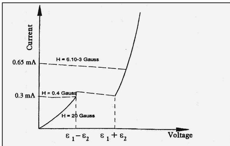
**Figure 2.** The current-voltage ( $I$ - $V$ ) characteristics observed by Anderson and Rowell showing the effect of magnetic field on the zero voltage current. In the earth's magnetic field ( $\sim 0.4$  Gauss) the current was  $0.3$  mA which increased to  $0.65$  mA when the junction was shielded by a mu-metal container. Also shown in the figure by the solid line is the curve when  $20$  Gauss field destroys the effect.
