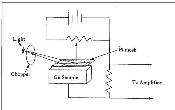
*Figure 2. Brattain's experiment to measure changes in contact potential due to light.*
