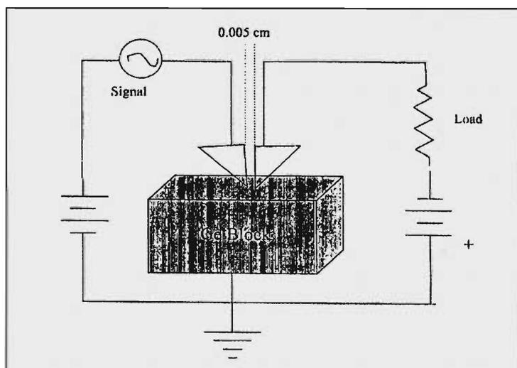
*Figure 4. Sketch of the arrangement in which the full transistor effect was first observed .*
