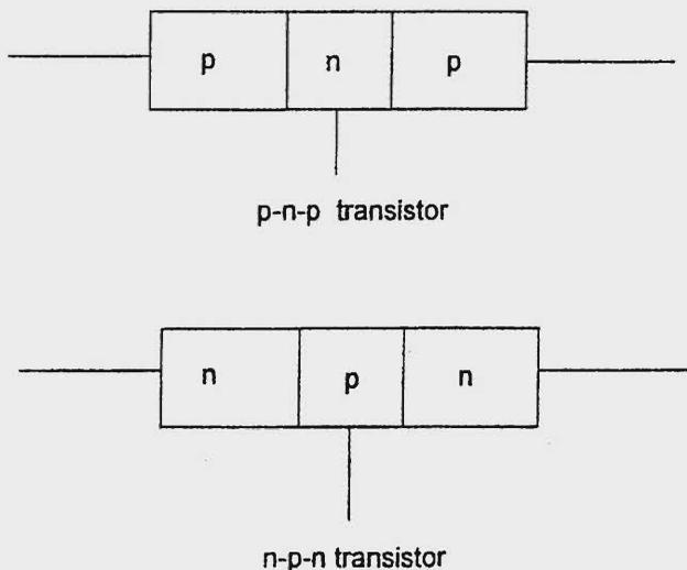
**Schematic representation of a p-n-p and an n-p-n transistor.**
