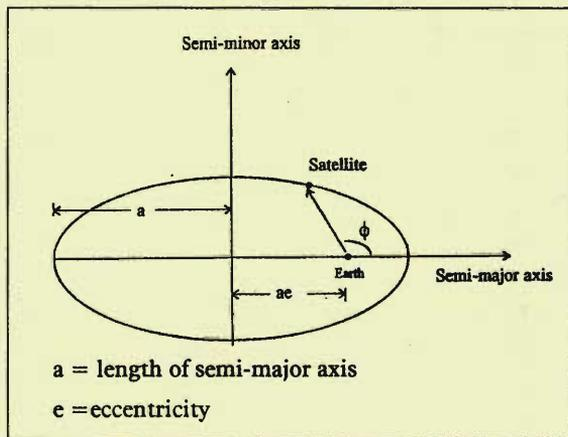
**Figure c. Elliptical orbit of a satellite.**
