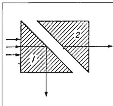
**Figure 1. Experiment to prove that Hertz waves enter the rarer medium. The distance between the two prisms is a fraction of the wavelength.**
