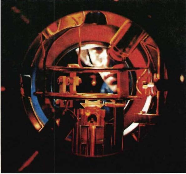
*Figure 4. A magneto-optical trap (MOT). The yellow dot is the cloud of sodium atoms. (Courtesy: Royal Swedish Academy of Sciences).*
