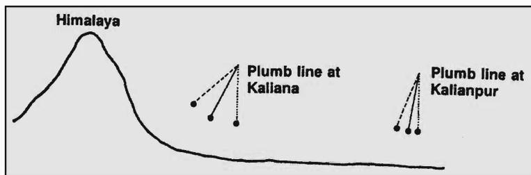
plumb line towards the Himalaya by about  $27''.853$  at Kaliana and about  $11''.968$  at Kalianpur. Thus the discrepancy between geodetically and astronomically estimated latitude should have been  $15''.805$ , nearly three times the observed value of  $5''.236$ . This meant that the Himalaya did not exert as much gravitational attraction on the plumb bobs as anticipated from their external massive appearance. It was as if the Himalayas were hollow inside.
