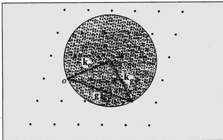
**Figure 1.** Ewald construction to show the diffraction phenomena.
