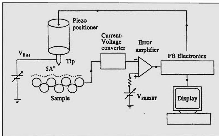
result for a given bias the current through the tunnel resistor decreases exponentially as the separation between the tip and the substrate increases. An STM uses this sensitive dependence of the tunnel current between the tip and the substrate to achieve the super resolution.
