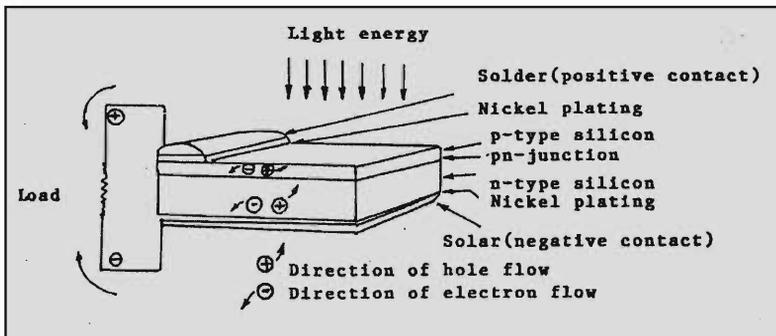
A photovoltaic cell consists of a p-n junction of a semiconductor. When light is incident electron-hole pairs are generated which diffuse to the two sides of the junction generating an open circuit voltage.
