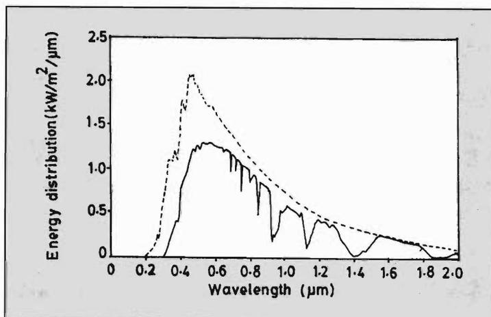
*Figure 2. Spectrum of the solar radiation. The area between the dashed line and solid line represents the portion of sunlight absorbed by the earth's atmosphere.*
