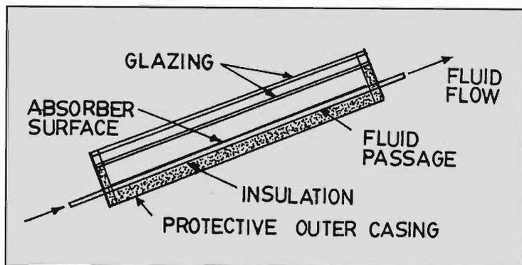
*Figure 4. A flat plate solar collector.*
