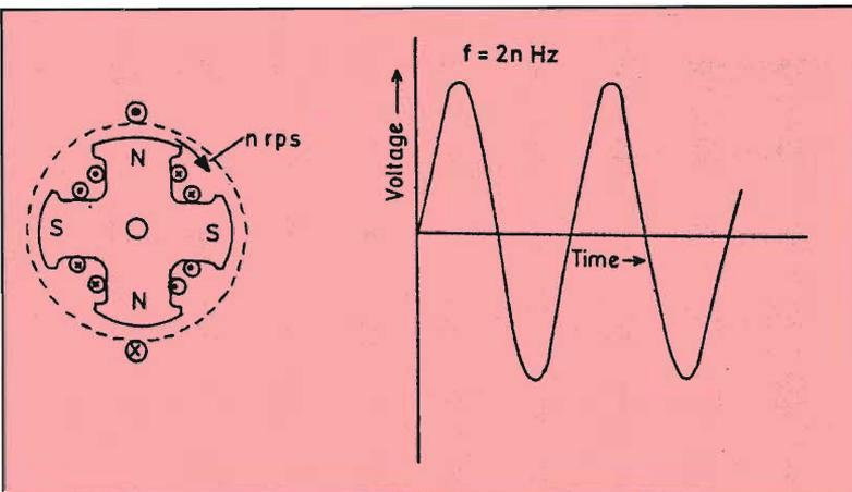
turbine is a huge cylinder of solid steel and it is wound in a manner that it produces two poles (some times, but seldom, four poles). Since 50 Hz power supply is used in India and also in Europe, the turbine has to be rotated at 50 rps (3000 rpm) for the frequency of the alternating voltage to be
