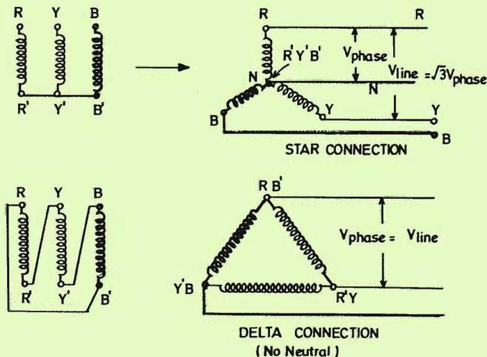
**Figure 8** Three phases can be connected either in star (Y) or as Delta ( $\Delta$ ). In star connection the line and phase currents are one and the same. But the line to line voltage is  $\sqrt{3}$  times the voltage between a line (or phase) and the neutral. In domestic connections a wire from the neutral and any one of the phases are brought in.
