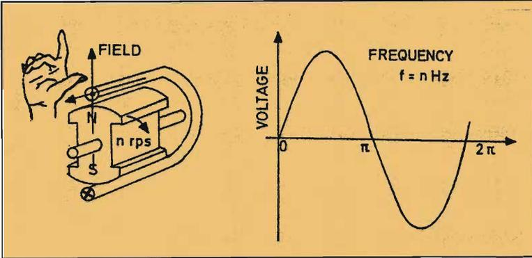
**Figure 3** When a magnet (electromagnet) is rotated inside a coil (in reality a set of coils) the magnetic field keeps changing its direction. The voltage/current in the coil correspondingly changes direction or alternates. (Fleming's right hand rule).
