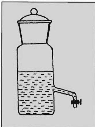
**Figure 3. Liquid weighing bottle. It has a side-arm with a stop-cock for draining a liquid. There is a hole in the neck and another hole in the hollow stopper. These two holes are made concentric by turning the stopper for drawing the liquid through the stop-cock. The bottle is weighed before and after drawing the liquid into a receiver to know the weight of the liquid drawn.**
