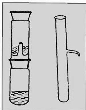
**Figures 4&5 (left) Micro distillation unit for liquids of a few ml quantity (right) Micro distillation tube for liquids less than 1 ml.**
