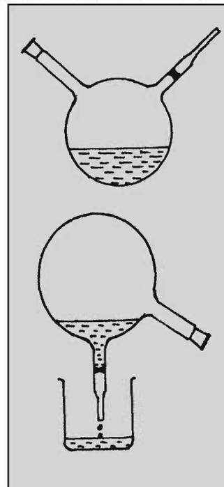
**Figure 2 Two-necked flask for small-scale crystallization and hot filtration. It has a sinter fused into one arm. This is suitable for a variety of organic laboratory operations, to be used with an air condenser, a Liebig condenser or as such.**
