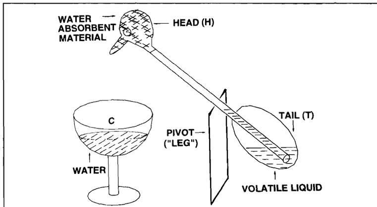
Figure 1 Schematic diagram of the thirsty bird.
