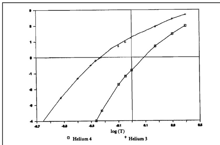
*Figure 3 Vapour pressure curves of liquid  $^3\text{He}$  and liquid  $^4\text{He}$ .*
