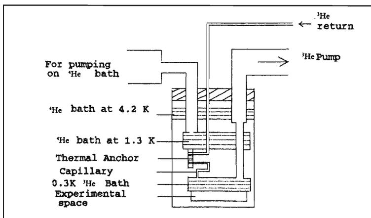
*Figure 4* A schematic diagram of a continuously operating liquid  $^3\text{He}$  cryostat to reach down to 0.3 K.
