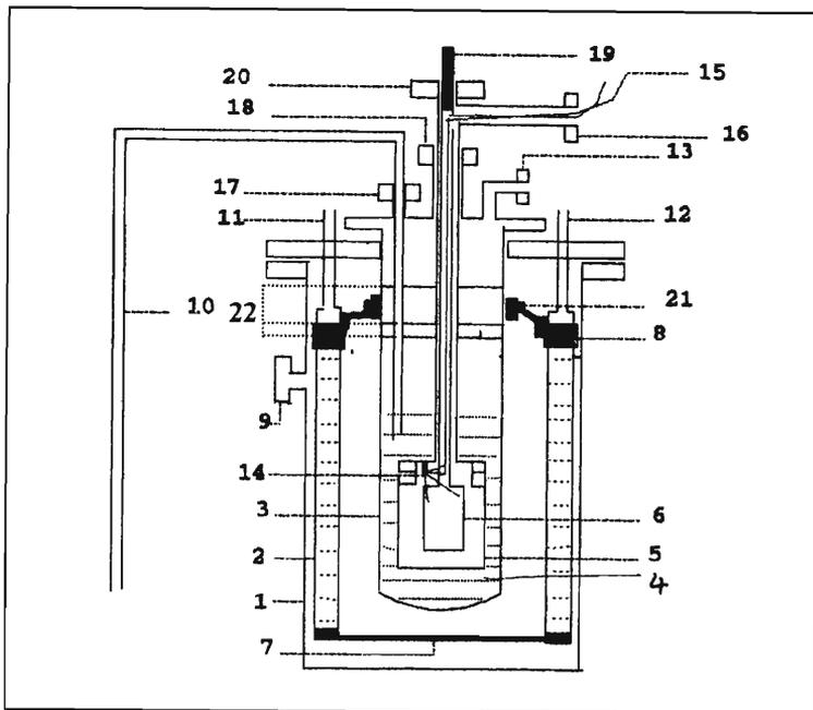
*Figure 2 A typical cryostat for measurement of electrical resistivity in the range 1.8 to 300 K.*
