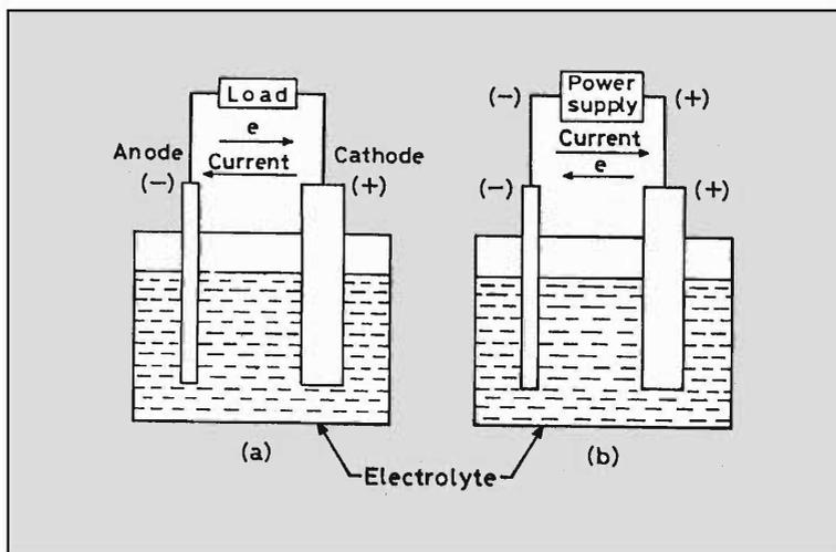
That is, they use chemical reactions to produce electricity. Such electrochemical devices are called *galvanic cells* in contrast to *electrolytic cells* which consume electrical energy to bring about a chemical reaction.
