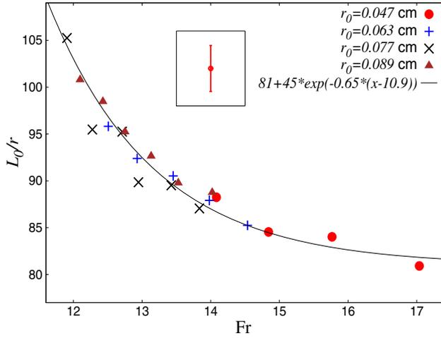
**Figure 6.** Plot of the dimensionless length  $L_0/r$  as a function of the Froude number  $Fr$ . Each point on the graph corresponds to a combination of parameters  $r_0$  and  $Q$  given in table 2. A typical length of the error bars is separately shown in the graph. The line is arbitrarily drawn to guide the eye.
