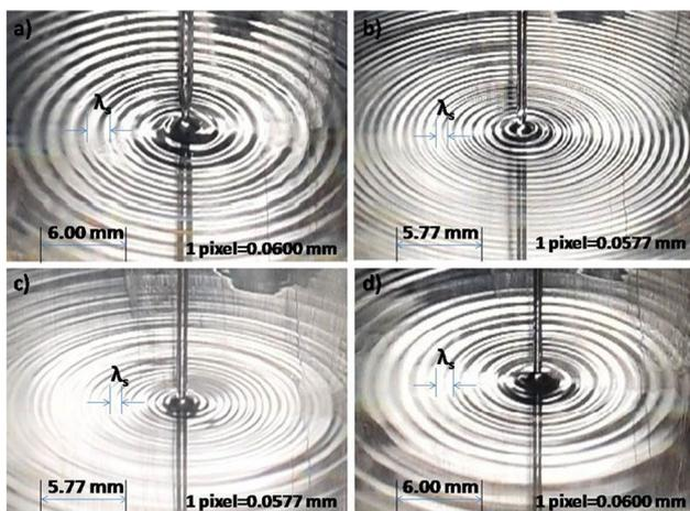
**Figure 2.** Photograph of waves on clean water ( $c = 0 \text{ mg cm}^{-3}$ ) reservoir surface at jet lengths (a)  $L = 0.168 \text{ cm}$ , (b)  $L = 0.568 \text{ cm}$ , (c)  $L = 3.618 \text{ cm}$  and (d)  $L = 4.268 \text{ cm}$ . The experimental parameters are:  $r_0 = 0.047 \text{ cm}$  and  $Q = 0.833 \text{ cm}^3 \text{ s}^{-1}$ .
