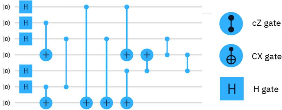
**Figure 6.** Quantum Circuit for the generation of the seven-qubit genuinely entangled state, on *IBM Quantum Experience*. Here *CX gate* is the CNOT gate, *cZ gate* is the CPHASE gate and *H gate* is the Hadamard gate.
