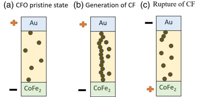
**Figure 5.** Bipolar resistive switching mechanism.
