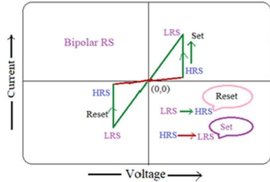
Figure 3. Bipolar resistive switching cycle.
