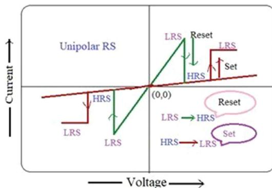
Figure 2. Unipolar resistive switching cycle.
