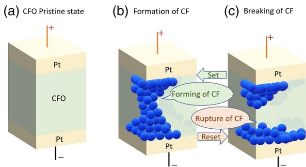
**Figure 4.** Formation and breaking of the conducting filament.
