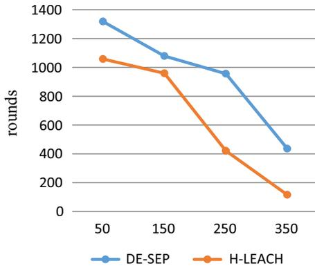
**Figure 2.** Stability period vs. rounds for increase in the base station distance from the centre of the network (50, 50), (50, 150), (50, 250) and (50, 350).
