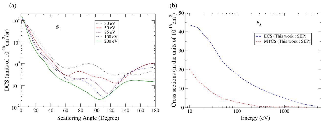
**Figure 6.** Cross-sections for  $e^-$  scattering of  $S_3$ . (a) Elastic DCS at 30 eV; dotted lines, 50 eV; dashed lines, 75 eV; dashed dotted lines, 100 eV; double dotted dashed lines and 200 eV; solid lines. (b) ECS; dashed lines and MTCS; dashed dotted lines.
