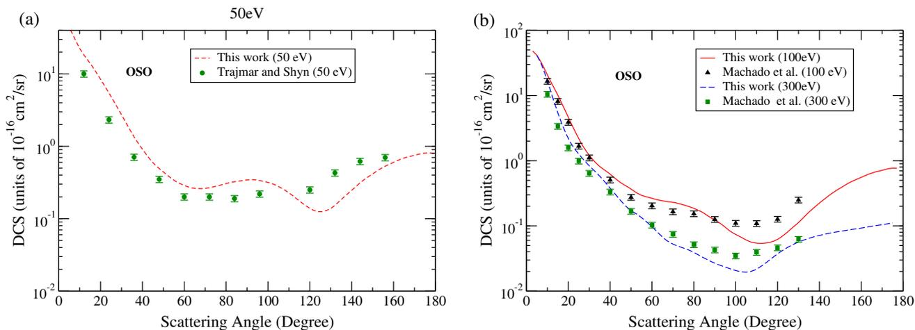
**Figure 9.** Elastic DCS for  $e^-$  scattering of OSO at (a) 50 eV and (b) 100 eV and 300 eV. Solid and dashed lines indicate this work, circles indicate the work of Trajmar and Shyn, triangles and squares indicate the work of Machado *et al*.
