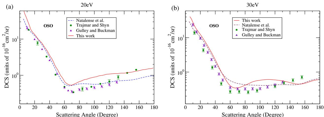
**Figure 8.** Elastic DCS for  $e^-$  scattering of OSO at (a) 20 eV and (b) 30 eV. Solid lines indicate this work, dashed lines indicate the work of Natalense *et al*, circles indicate the work of Trajmar and Shyn and triangles indicate the work of Gulley and Buckman.
