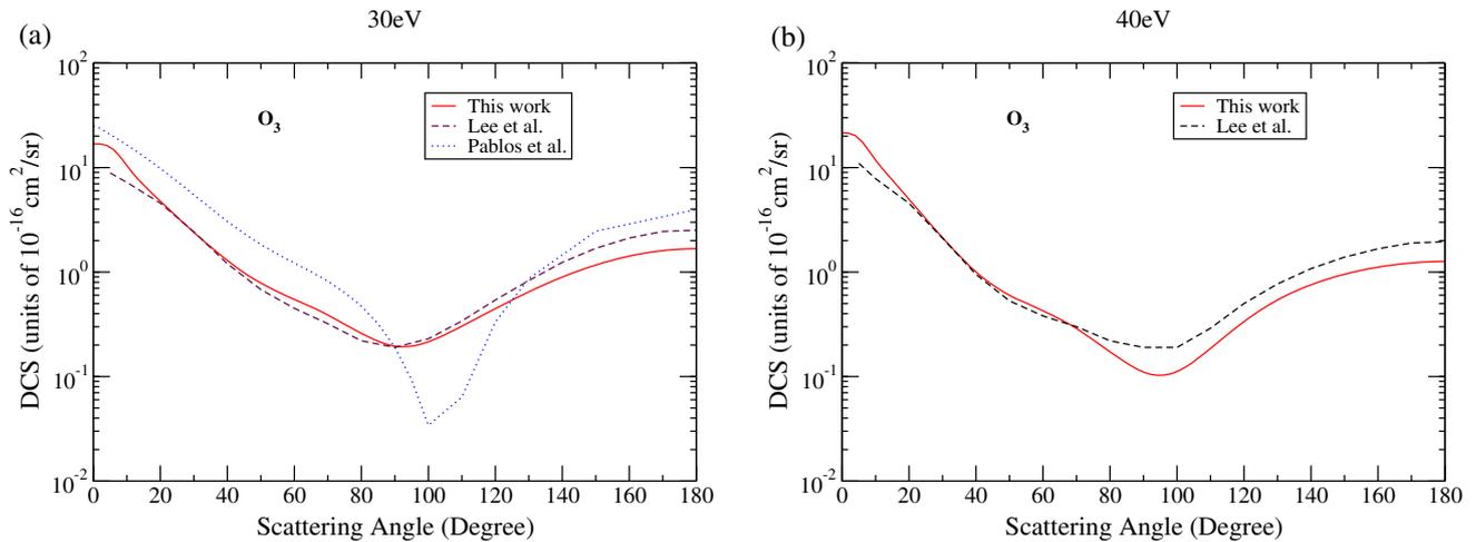
**Figure 2.** Same as figure 1 but at 30 eV and 40 eV. Solid lines indicate this work, double dashed lines indicate the work of Lee *et al* and dotted lines indicate the work of Pablos *et al*.
