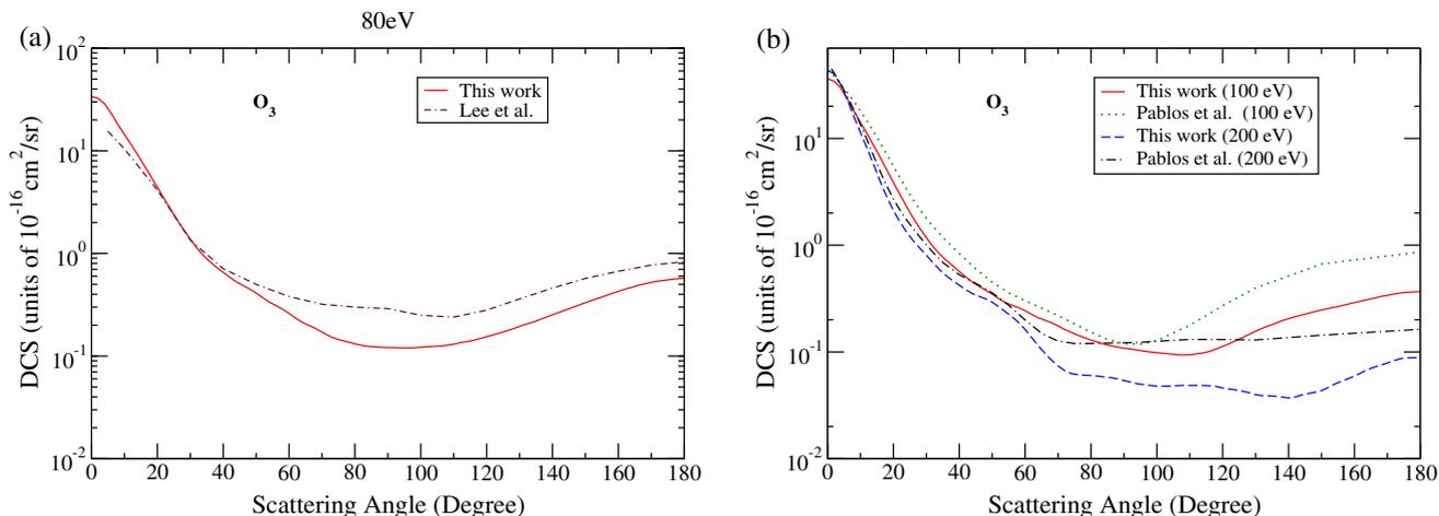
**Figure 4.** Elastic DCS at (a) 80 eV, (b) 100 eV and 200 eV. Solid and dashed lines indicate this work, dashed dotted lines indicate the work of Lee *et al* and dotted and dashed dotted lines indicate the work of Pablos *et al*.
