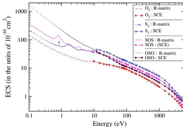
**Figure 14.** ECS for the isovalent molecules from the amalgamation of R-matrix and SCE formalisms.
