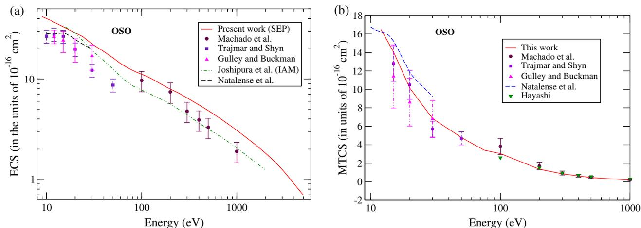
**Figure 11.** Cross-sections for  $e^-$  scattering of OSO. (a) ECS and (b) MTCS. Solid lines indicate his work, double dotted dashed line indicates the work of Joshipura *et al.*, dashed lines indicates the work of Natalense *et al.*, triangles indicate the work of Gulley and Buckman, squares indicate the work of Trajmar and Shyn, circles indicate the work of Machado *et al.* and inverted triangles indicate the work of Hayashi.
