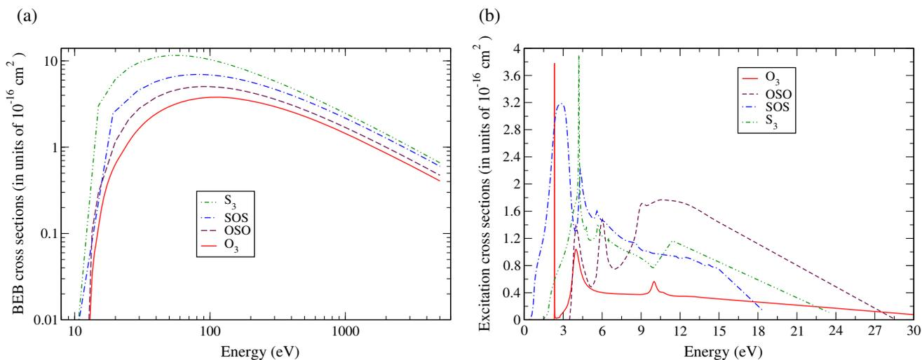
**Figure 16.** Inelastic cross-sections of isovalent targets. (a) BEB ionisation and (b) electronic excitation.
