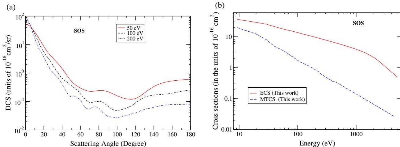
**Figure 12.** Cross-sections for  $e^-$  scattering of SOS. (a) Elastic DCS at 50 eV (solid line), 100 eV (dashed line) and 200 eV (double dotted dashed line) and (b) ECS (solid line) and MTCS (dashed line).
