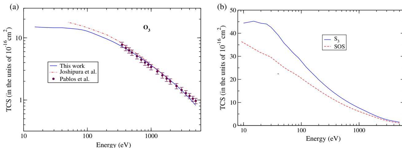
**Figure 17.** TCS for (a)  $O_3$ : solid line indicates this work, dashed double dotted line indicates Joshiyura *et al.*, circles indicate Pablos *et al.* and (b)  $S_3$  (solid line; this work) and SOS (dashed double dotted line; this work).
