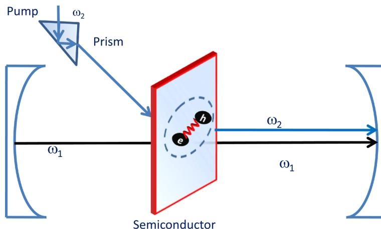
**Figure 1.** Block diagram of photon–exciton interaction in a cavity. The semiconductor crystal is put in a cavity filled with radiation.
