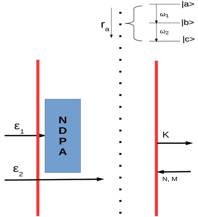
**Figure 1.** Schematic representation of non-degenerate three-level laser with a non-degenerate parametric amplifier (NDPA) and coupled to a two-mode squeezed vacuum reservoir. Here,  $\varepsilon_1$  is a real constant proportional to the amplitude of the pump mode that drives the NDPA while  $\varepsilon_2$  describes the amplitude of the coherent light. In addition,  $r_a$  is the rate of atomic injection into the cavity and  $\kappa$  (kappa) is the cavity damping constant.
