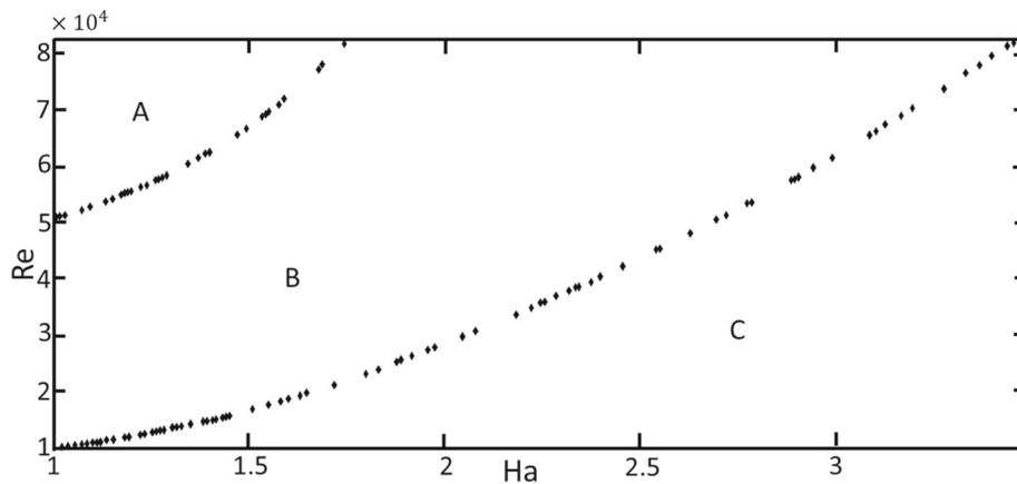
Figure 7. Streamwise instability curves for  $k = 1$ .
