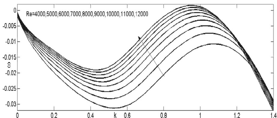
Figure 5. Growth rate curves  $\omega$  with  $k$  for various values of  $Re$ .
