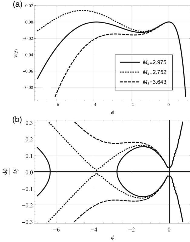
**Figure 3.** For large amplitude DLs, (a) plot of  $V(\phi)$  vs.  $\phi$  for different Mach numbers  $M_s$  with  $\alpha = 5$ ,  $\beta = 0.2$ ,  $\theta = 50$  and  $q = 0.69$  and (b) the corresponding phase portrait.
