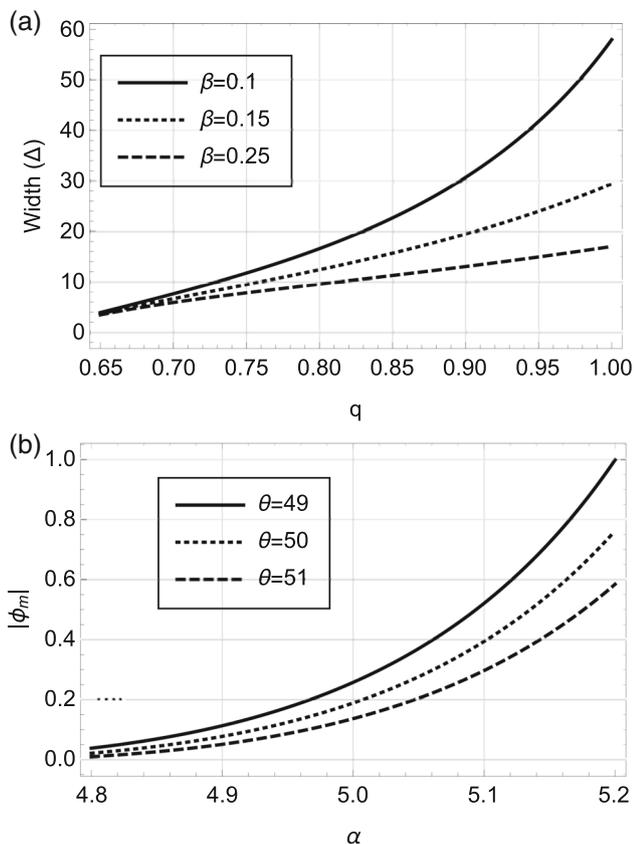
**Figure 6.** For  $\alpha = 5$  and  $\theta = 50$ , variation of (a) width of DL as a function of  $q$  for different values of  $\beta$  with  $M = 2.7$  and (b) amplitude  $|\phi_m|$  vs.  $\alpha$  for different values of  $\theta$  with  $M = 2.6$ .
