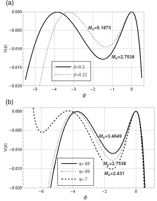
**Figure 4.** Sagdeev potential  $V(\phi)$  vs.  $\phi$  (a) for different values of  $\beta$  with  $\theta = 50$  and  $q = 0.69$  and (b) different values of non-extensive parameter  $q$  with  $\alpha = 5$ ,  $\beta = 0.2$ .
