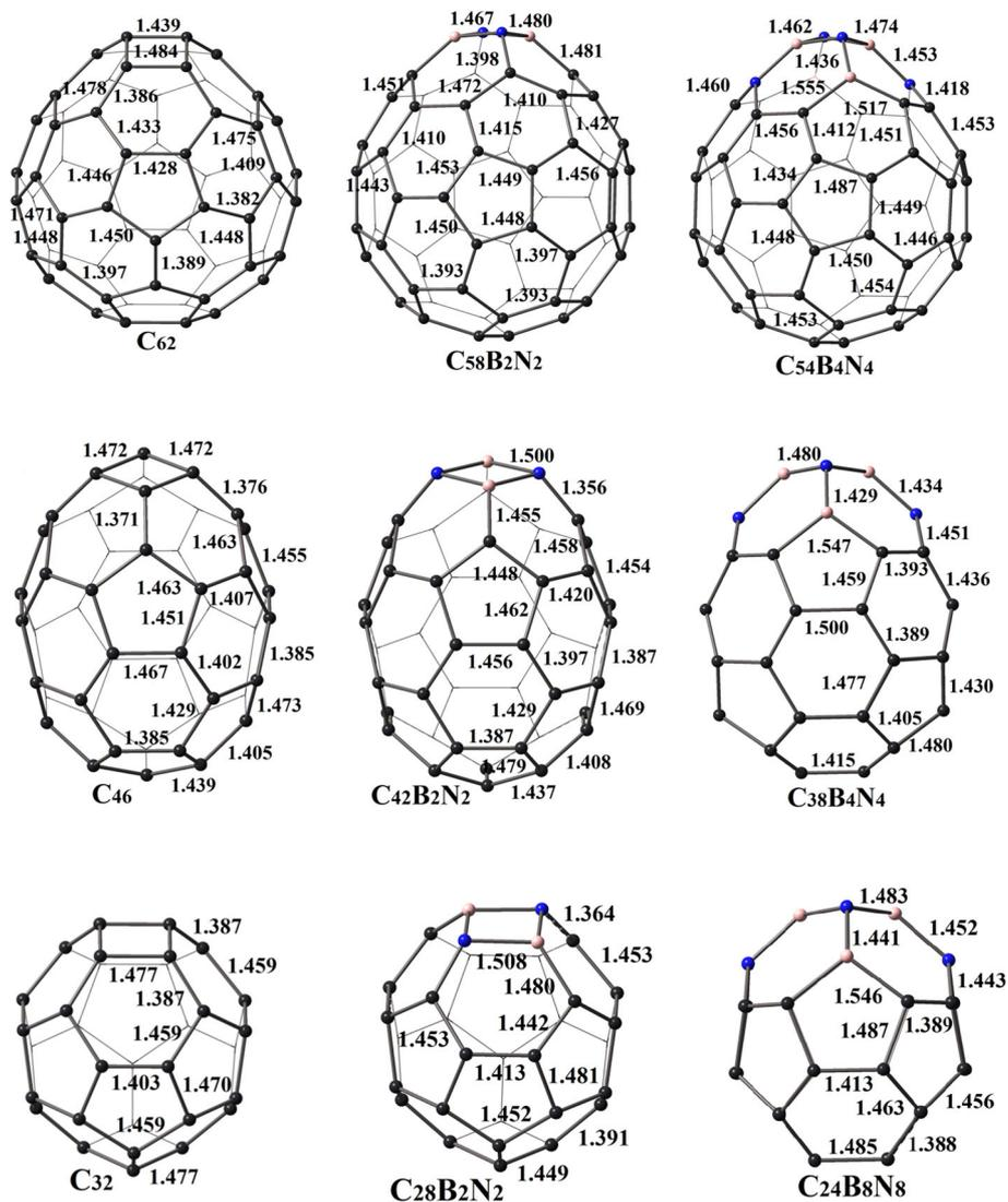
**Figure 2.** The optimised geometries of the BN-substituted non-IPR fullerenes together with their parents. The geometrical parameters (in Å) are shown.
