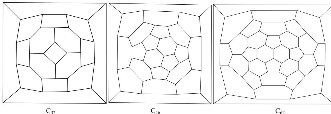
**Figure 1.** Schlegel diagrams of the non-IPR fullerenes,  $C_{62}$  and  $C_{46}$  with one square ring and  $C_{32}$  with two square rings.
