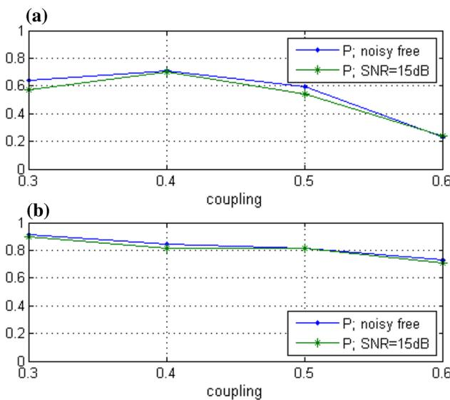
**Figure 3.** Peak value  $P$  of MSC between time series of the master oscillator and  $\hat{S}(t)$  for two unidirectionally coupled Rössler systems in the phase synchronisation regime with a locking rate of 1:4 (a) at the intrinsic frequency of the drive oscillator and (b) at the second harmonic of the drive signal.
