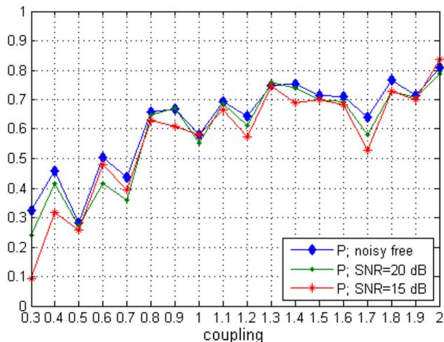
**Figure 4.** Peak value  $P$  of MSC between the time series of the master oscillator and  $\hat{S}(t)$  for two unidirectionally coupled Van der Pol oscillators.
