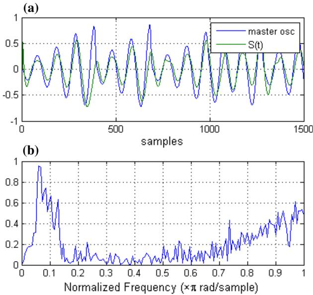
**Figure 1.** (a) Time series of the master oscillator and  $\hat{S}(t)$  and (b) magnitude squared coherence between time series of the master oscillator and  $\hat{S}(t)$ .
