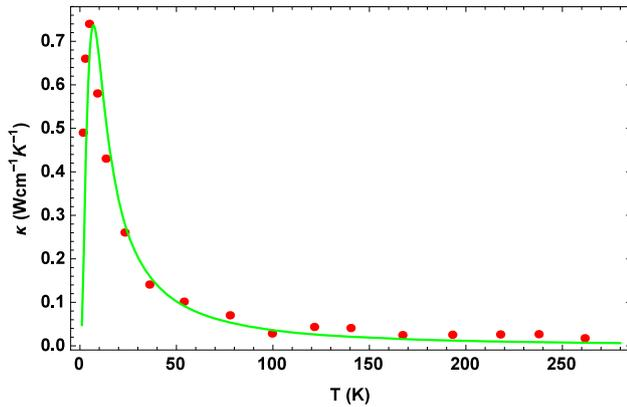
**Figure 2.** Thermal conductivity of the PbS semiconductor. The dots represent the experimental data and the thick line depicts theoretical results.
