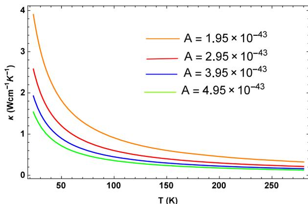
**Figure 1.** Effect of mass change parameter on the thermal conductivity of the PbS semiconductor.
