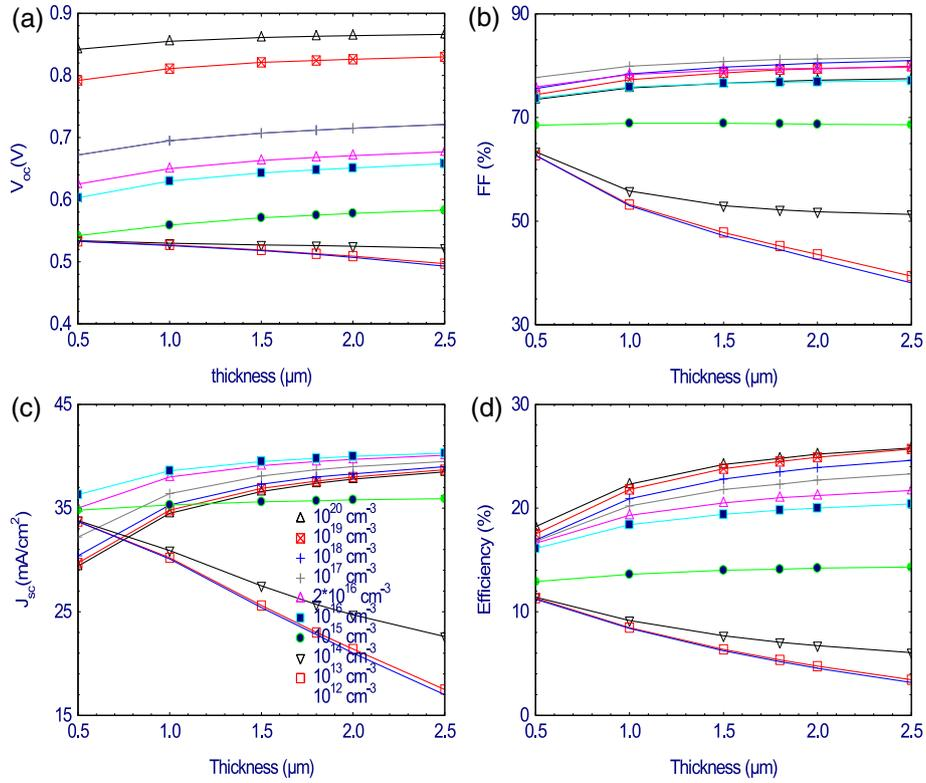
Figure 3. Variation of the electrical parameters with respect to the thickness according to the doping concentration.
