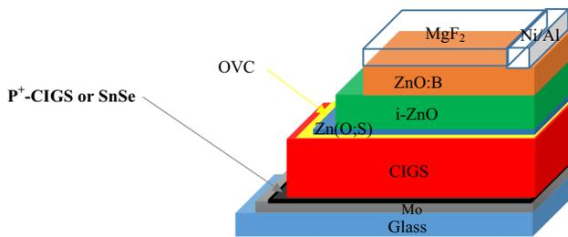
**Figure 9.** Structure of the CIGS-based solar cell with BSF.
