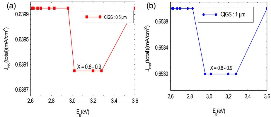
**Figure 8.** Variation of the total recombination current with the band-gap energy.
