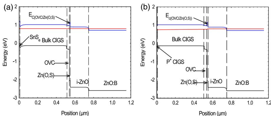
**Figure 12.** Band energy diagram of the structure with (a) SnSe and (b) p<sup>+</sup>-CIGS as BSF.
