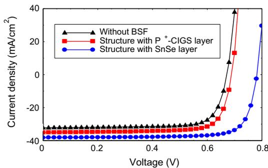
**Figure 10.** Current–voltage characteristics of the structures without and with different BSF layers.
