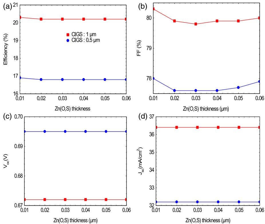
Figure 4. Influence of Zn(O,S) thickness on the electrical parameters according to the CIGS thickness.
