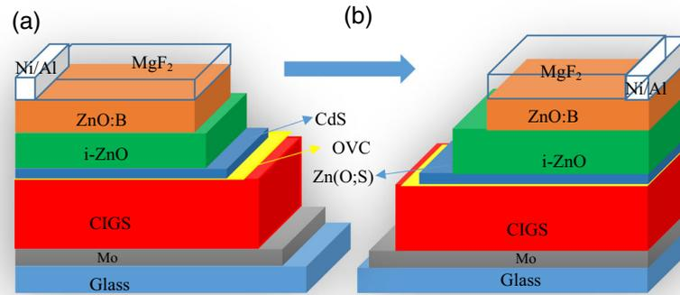
**Figure 1.** Structures of CIGS-based solar cell used in the simulation: the CdS layer is replaced by a Cd-free layer.
