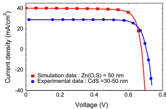
**Figure 2.** Comparison of current–voltage simulation curve with experimental data of ref. [1].
