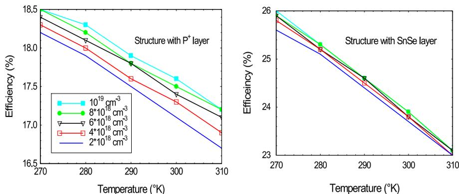
**Figure 11.** Variation of efficiency with temperature and doping concentration of the BSF.
