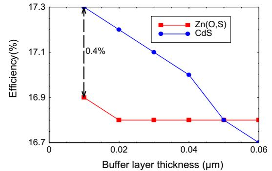
**Figure 5.** Comparison of efficiencies of CIGS cells buffered Zn(O,S) and CdS at 0.5  $\mu$ m absorber thickness.
