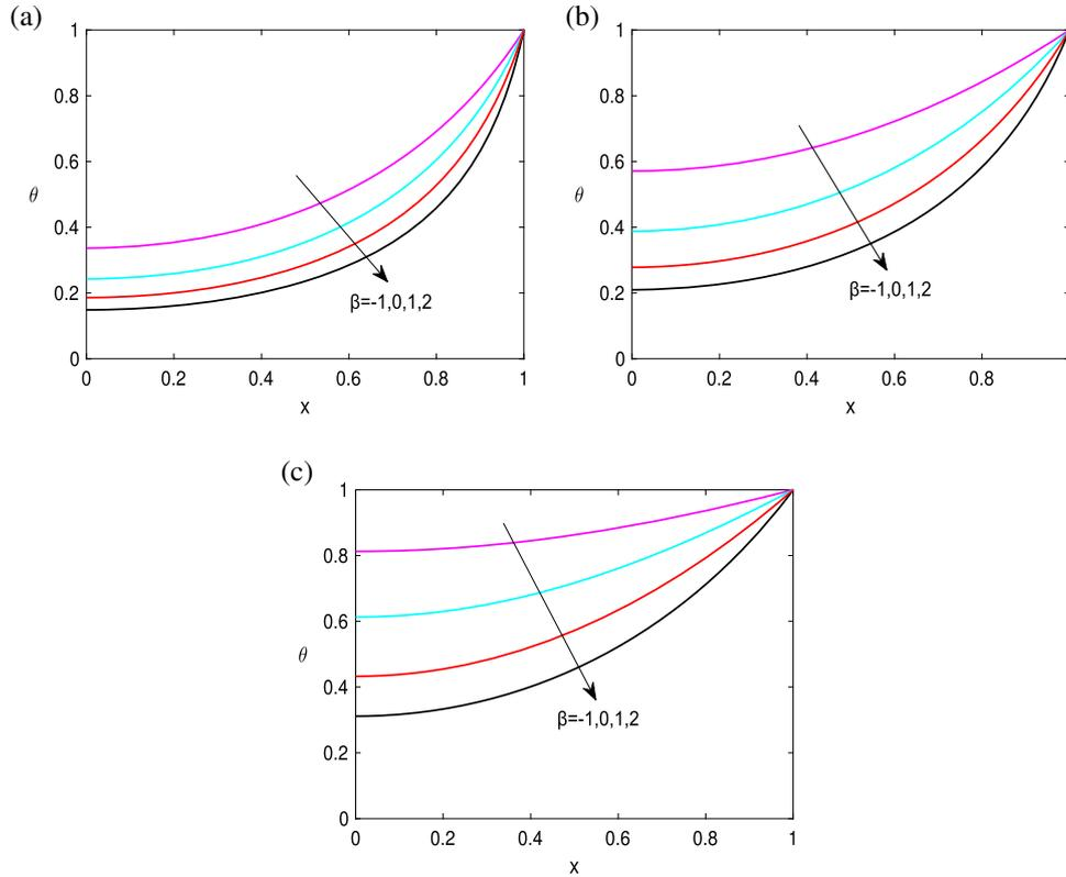
**Figure 3.** The dimensionless temperature excess  $\theta$  for  $M = 1.6$  and different values of  $\beta$ . **(a)**  $\alpha = -1$ , **(b)**  $\alpha = 0$  and **(c)**  $\alpha = 1$ .
