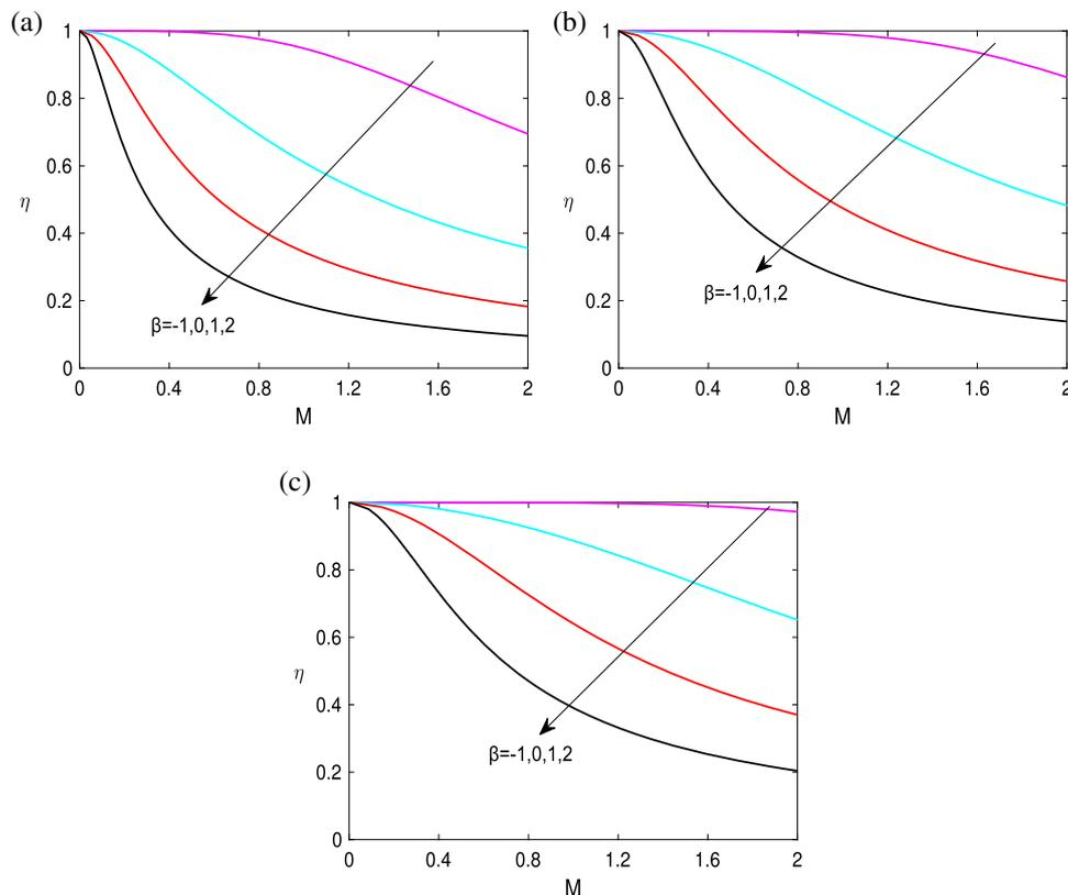
**Figure 7.** The fin efficiency against  $M$  for different values of  $\beta$ . (a)  $\alpha = -1$ , (b)  $\alpha = 0$  and (c)  $\alpha = 1$ .
