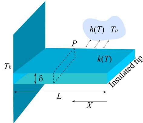
**Figure 1.** Schematic of a convective fin with rectangular cross-section along with coordinates.
