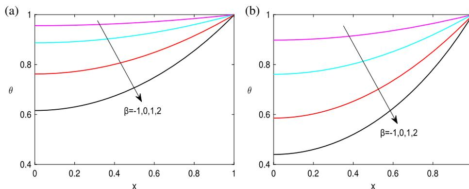
**Figure 5.** The dimensionless temperature excess  $\theta$  for  $\alpha = 1$  and different values of  $\beta$ . (a)  $M = 0.8$  and (b)  $M = 1.2$ .
