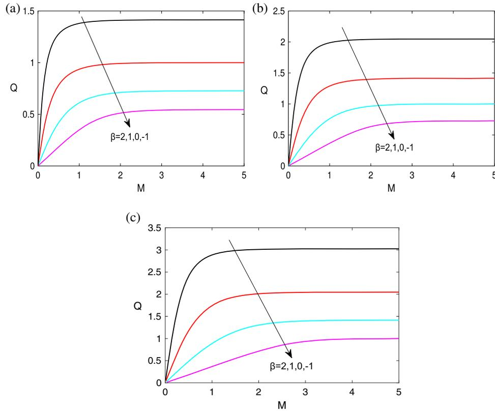
**Figure 6.** The dimensionless fin heat transfer rate against  $M$  for different values of  $\beta$ . (a)  $\alpha = -1$ , (b)  $\alpha = 0$  and (c)  $\alpha = 1$ .
