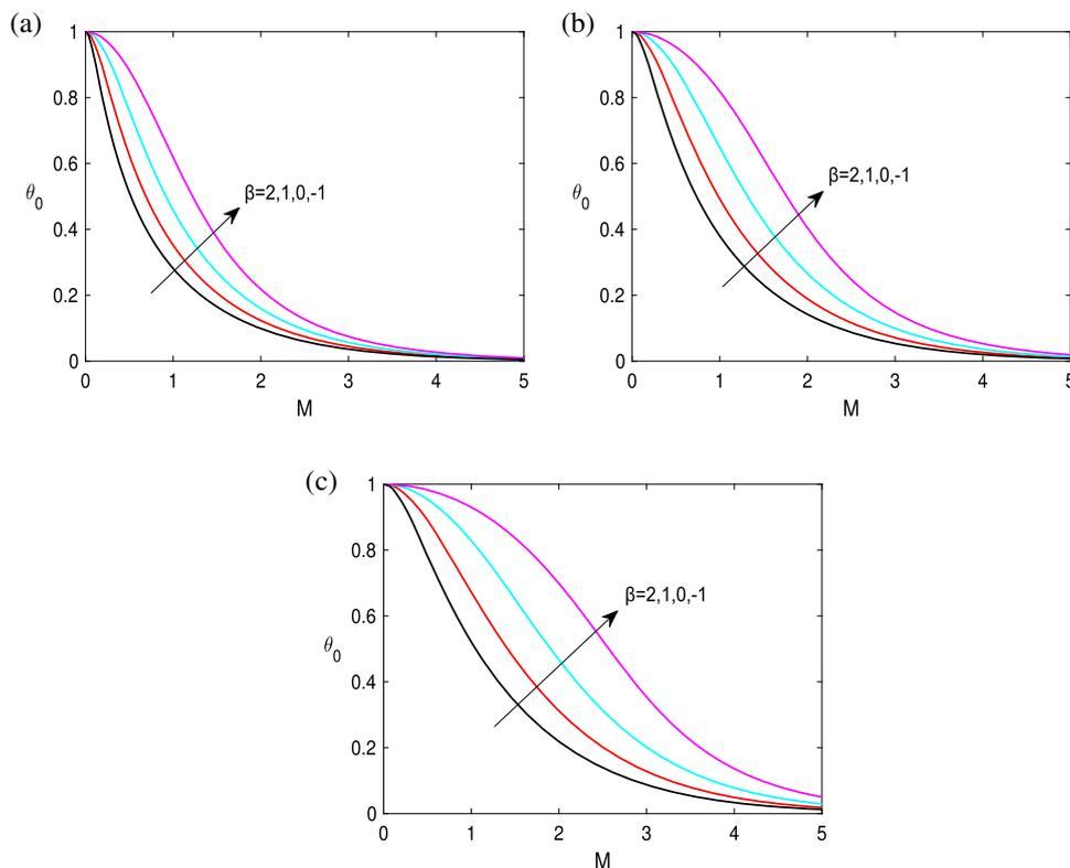
**Figure 2.** The dimensionless temperature value  $\theta_0$  at the fin tip for different values of  $\beta$ . (a)  $\alpha = -1$ , (b)  $\alpha = 0$  and (c)  $\alpha = 1$ .
