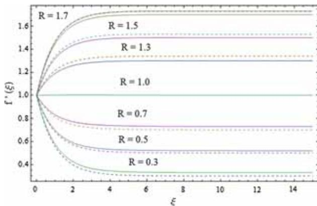
**Figure 8.** The effect of  $R$  on velocity profile.
