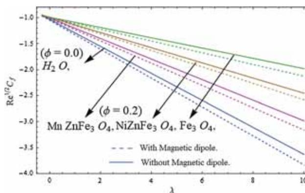
**Figure 10.** Influence of  $\phi$  on wall shear stress vs.  $\lambda$ .
