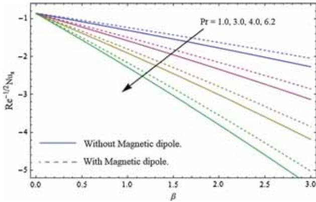
**Figure 12.** The influence of Pr on heat transfer rate vs.  $\beta$ .
