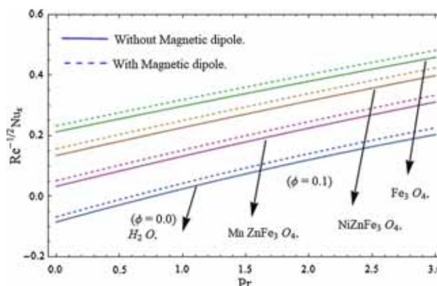
**Figure 11.** The influence of  $\phi$  on heat transfer rate vs.  $\text{Pr}$ .
