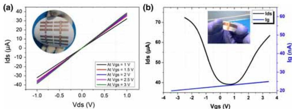
**Figure 3.** (a) Drain characteristics with the inset showing the array of fabricated devices and (b) transfer characteristics with gate leakage current of graphene FET (inset showing the fabricated device).
