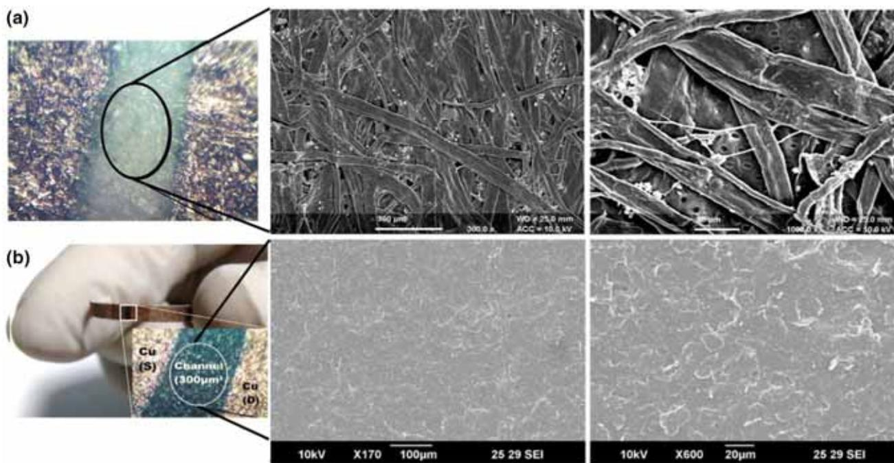
**Figure 2.** Pre-fabricated device with the source and the drain contact electrode (a) without and (b) with graphene active layer deposited in between (inset shows SEM image of the channel area).
