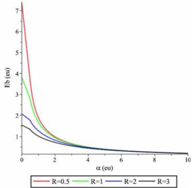
**Figure 1.** Binding energy of the exciton in GaAs vs. the field parameter  $\alpha$  for various radii of the quantum dot (e.u.).
