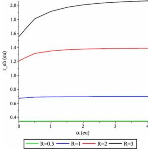
**Figure 2.** Variations of the spatial extension of the exciton ( $r_{eh}$ ) vs. the field parameter ( $\alpha$ ) for various radii of the dot in GaAs.
