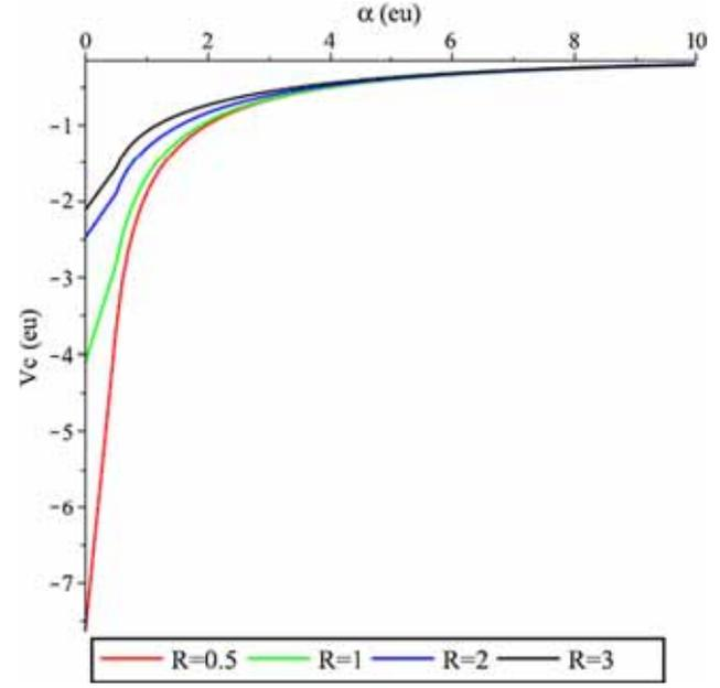
**Figure 3.** Dressed potential of the exciton vs. the field parameter ( $\alpha$ ) in GaAs quantum dot for various radii of the dot (e.u.)
