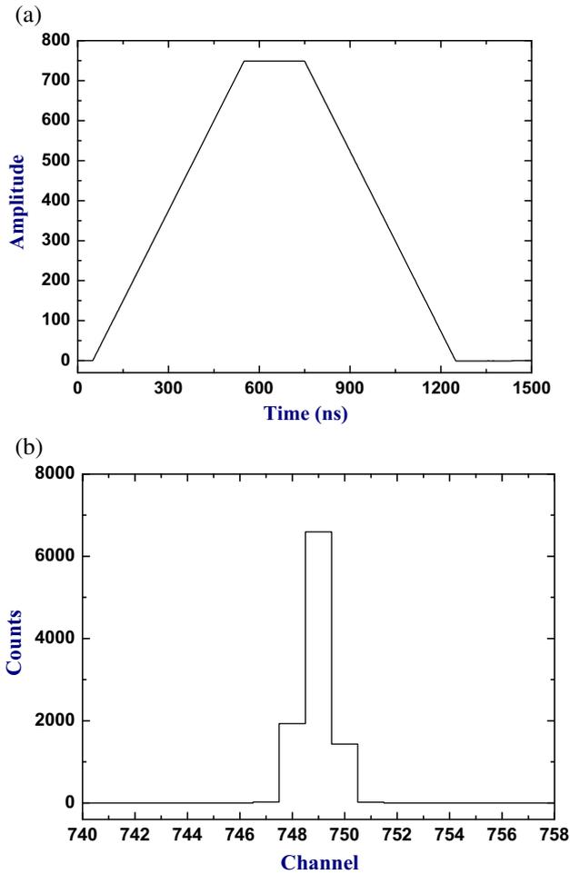
**Figure 2.** (a) Trapezoidal filtering of the pre-amplifier pulse and (b) the corresponding energy histogram after the shaping of the pre-amplifier signal.
