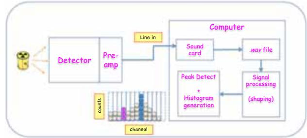
**Figure 3.** Schematic block diagram of the experimental set-up.
