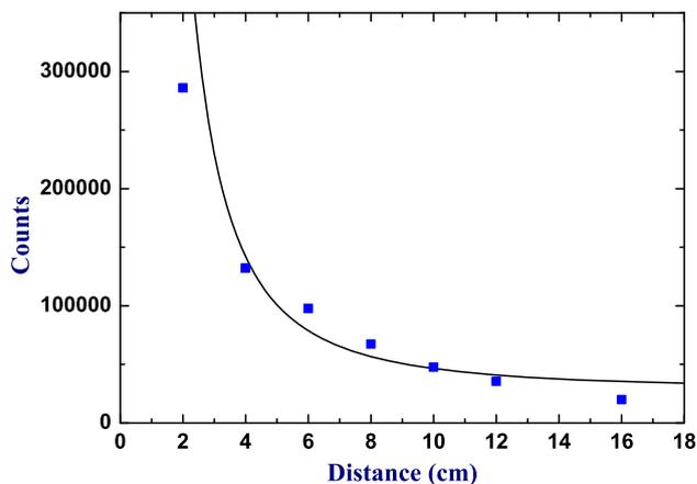
**Figure 6.** The observed counts for  $E_\gamma = 662$  keV as a function of the distance of the source from the detector face. The solid line presents the fit to  $y \propto 1/r^2$ .
