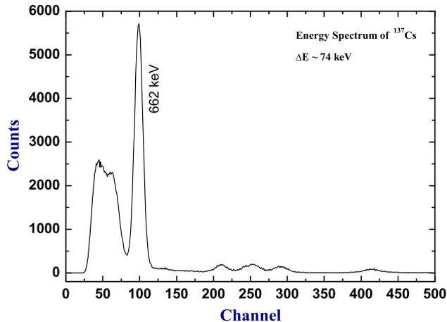
**Figure 5.** <sup>137</sup>Cs spectrum measured with the developed system.
