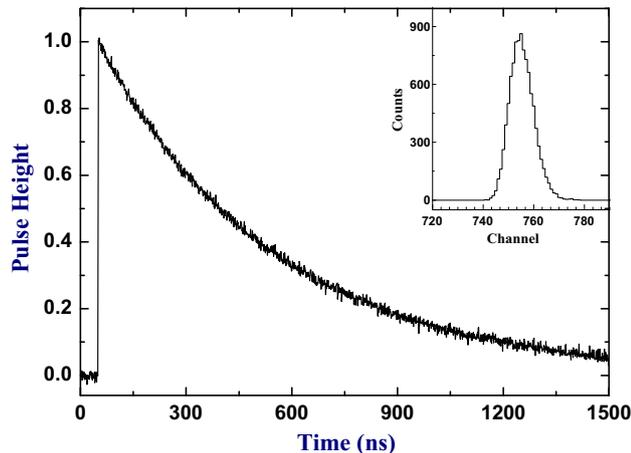
**Figure 1.** Simulated scintillator pulse for NaI(Tl), with SNR = 40 and the inset shows the corresponding energy histogram without the shaping of the pre-amplifier signal.
