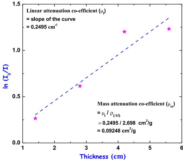
**Figure 7.** Plot of the observed attenuation for  $E_\gamma = 662$  keV as a function of the absorber thickness.
