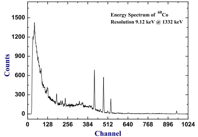
**Figure 8.**  $^{60}\text{Co}$  spectrum acquired with the present system using HPGc detector.
