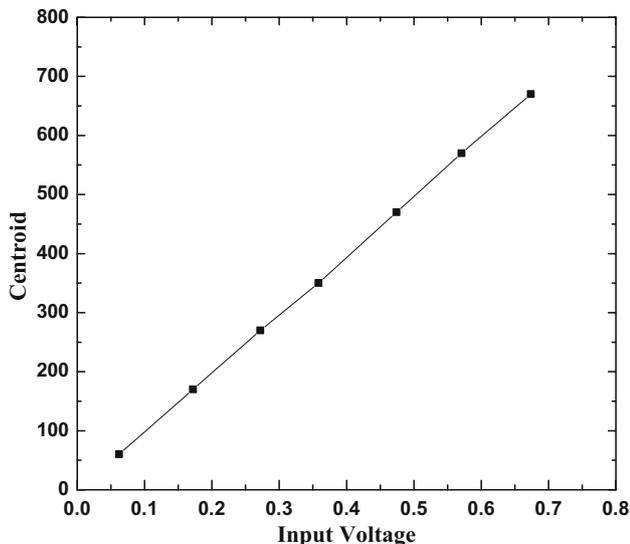
**Figure 4.** The observed correlation between the recorded peak centroid and the amplitude of the input voltage from a pulse generator recorded using the developed system.
