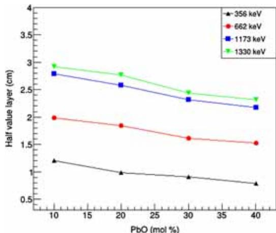
**Figure 8.** Dependence of HVL on the PbO fraction in the glasses.
