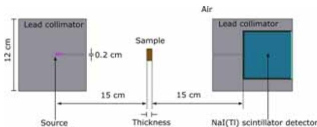
Figure 3. Schematic of the Fluka set-up.
