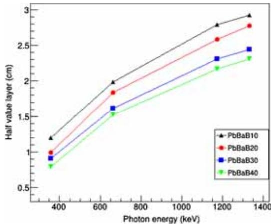
**Figure 7.** Half value layer of the PbBaB glass system as a function of photon energy.
