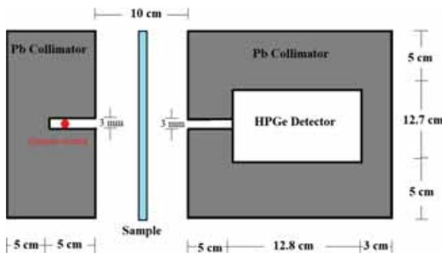
Figure 2. Schematic of the Geant4 set-up.
