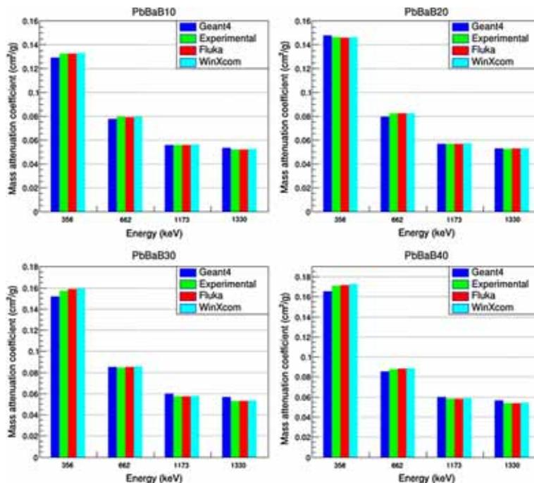
Figure 4. Comparison of the computationally determined  $\mu_m$  values with the experimental data.
