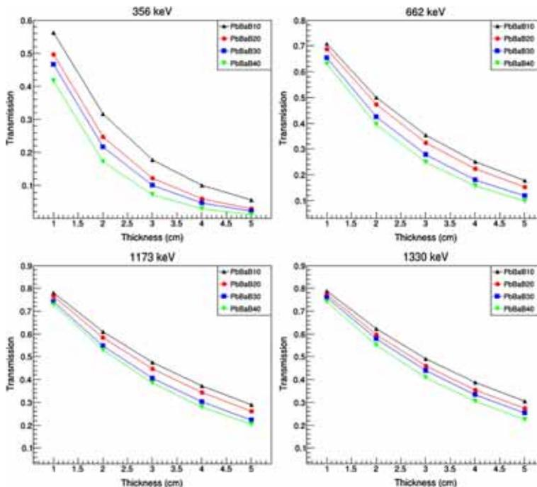
Figure 5. Transmission factor vs. thickness of PbBaB glass system at 356, 662, 1173 and 1330 keV photon energies.
