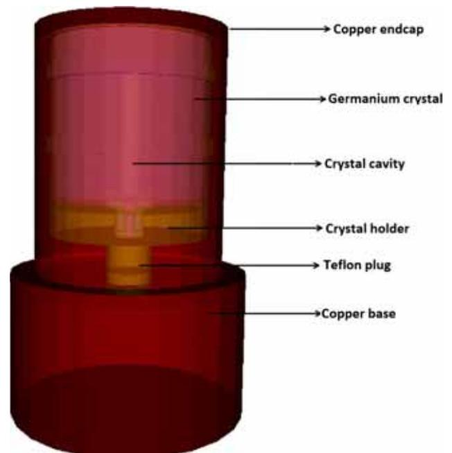
**Figure 1.** Geant4 model of the HPGe detector used for the determination of  $\mu_m$ .
