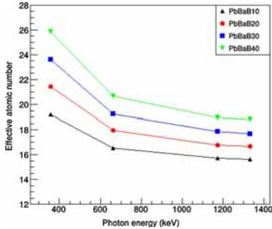
**Figure 6.** Variation of  $Z_{\text{eff}}$  with respect to photon energy for the PbBaB glass system.
