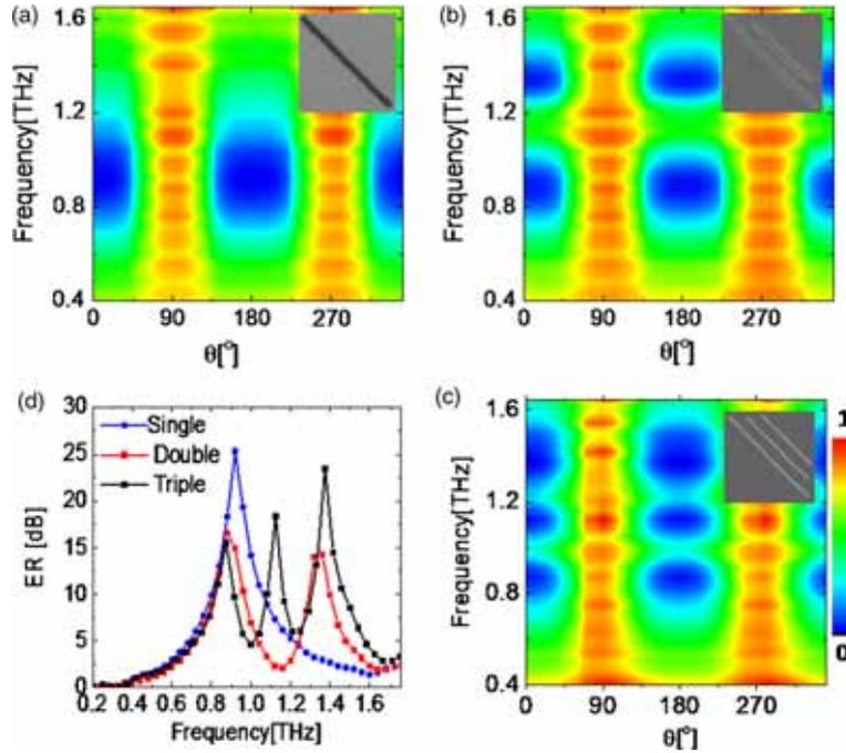
**Figure 5.** (a)–(c) The measured normalised transmission coefficient for single, double, and triple narrowband THz polarisers at 0.92 THz, (0.88, 1.36) THz and (0.87, 1.13, 1.37) THz, respectively and (d) The plot of ER as a function of frequency for all the three devices.
