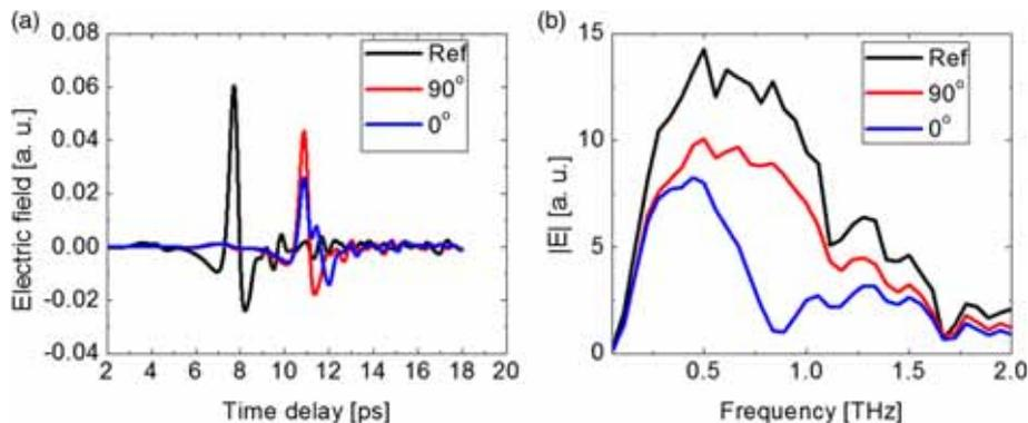
**Figure 3.** (a) THz waveforms transmitted through the reference, through the single cut-wire MM for angle  $\theta = 90^\circ$  and  $0^\circ$  and (b) amplitude of the electric field obtained by Fourier transformation of the reference and sample waveforms. We can see an absorption in the spectrum at 0.9 THz for  $\theta = 0^\circ$ .
