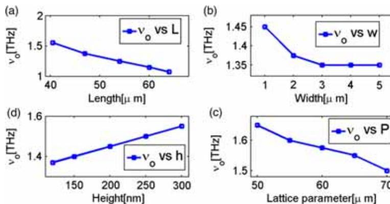
**Figure 2.** (a) Resonance frequency vs. length of the cut-wires from FEM simulations, (b) resonance frequency vs. width of the wires from FEM, (c) resonance frequency vs. lattice parameter from FEM simulation data, and (d) resonance frequency vs. height of the wires from FEM.
