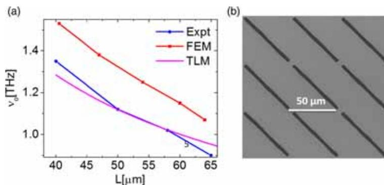
**Figure 4.** (a) Comparison of the centre frequency of resonance vs. length of the cut-wires from the experimental (Expt) data, FEM data, and TLM and (b) SEM image of the single-wire MM.
