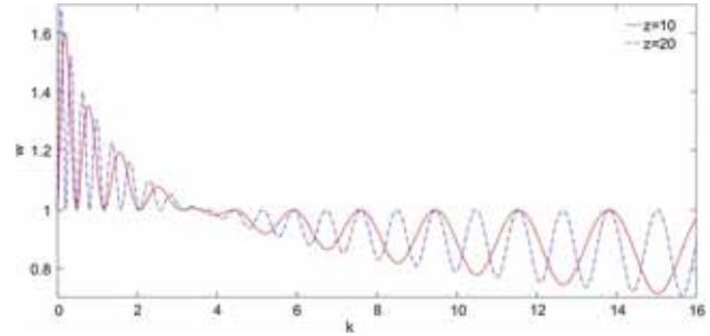
**Figure 4.** The variation of the width of the light beam with the trap frequency  $k$  when  $z = 10$  and  $20$ . The parameters  $w_0 = 1$  and  $s' = 0.1$ .
