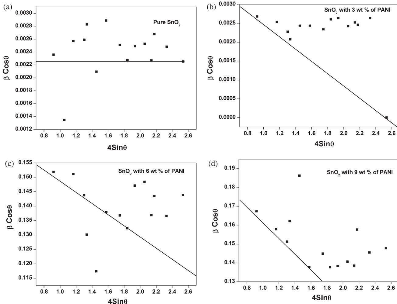
**Figure 2.** W–H plot of (a) pure  $\text{SnO}_2$ , (b) 3 wt%, (c) 6 wt% and (d) 9 wt% of PANI in the  $\text{SnO}_2/\text{PANI}$  nanocomposite.
