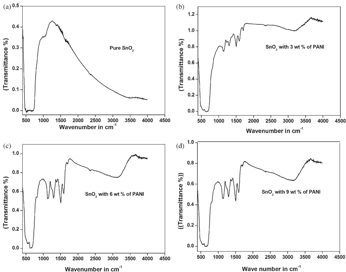
**Figure 4.** FT-IR spectra of (a) pure  $\text{SnO}_2$ , (b) 3 wt%, (c) 6 wt% and (d) 9 wt% of PANI in the  $\text{SnO}_2$ /PANI nanocomposite.
