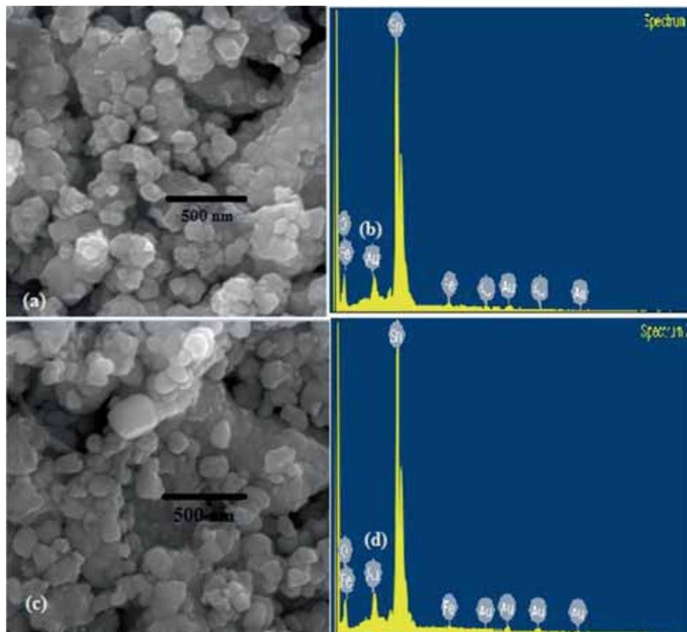
**Figure 3.** SEM image of (a) pure SnO<sub>2</sub>, (b) EDAX of pure SnO<sub>2</sub>, (c) SEM image of the SnO<sub>2</sub>/PANI nanocomposite and (d) EDAX of the SnO<sub>2</sub>/PANI nanocomposite.
