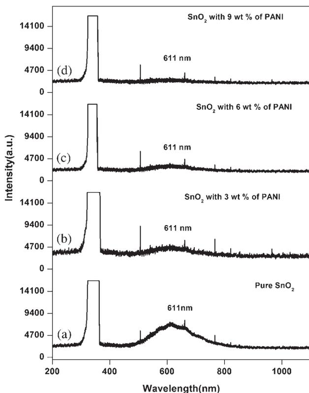
**Figure 5.** PL spectra of (a) pure SnO<sub>2</sub>, (b) 3 wt%, (c) 6 wt% and (d) 9 wt% of PANI in the SnO<sub>2</sub>/PANI nanocomposite.
