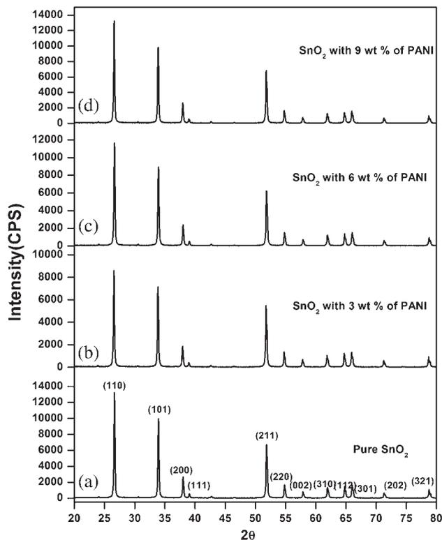
**Figure 1.** XRD patterns of (a) pure SnO<sub>2</sub>, (b) 3 wt%, (c) 6 wt% and (d) 9 wt% of PANI in the SnO<sub>2</sub>/PANI nanocomposite.
