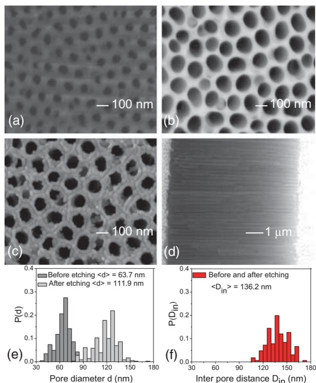
**Figure 1.** FESEM images of the NAA sample: (a) before etching, (b) after etching in phosphoric acid, (c) the gold-coated surface of the etched sample, (d) cross-sectional view of the gold-coated NAA, (e) distribution of pore diameters before and after etching and (f) distribution of inter pore distance before and after etching.
