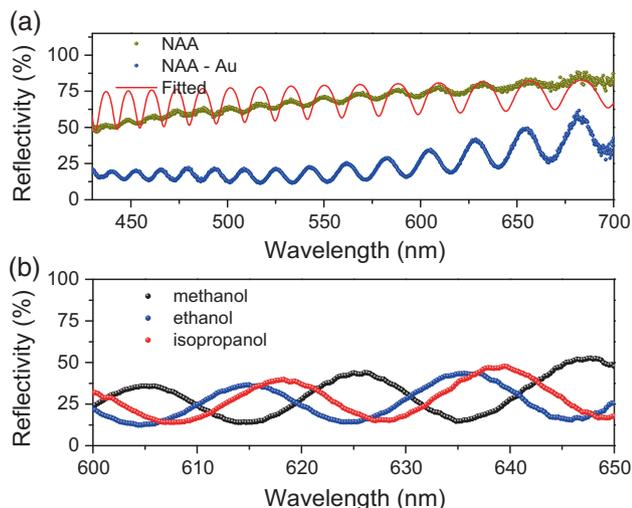
**Figure 3.** (a) Optical reflection spectrum of the NAA slab. Dark yellow curve: bare NAA slab, blue curve: NAA slab having a thin gold coating, and red curve: theoretical fit using TMM method and (b) reflectivity from gold-coated NAA membrane loaded with methanol (black curve), ethanol (blue curve) and isopropanol (red curve).
