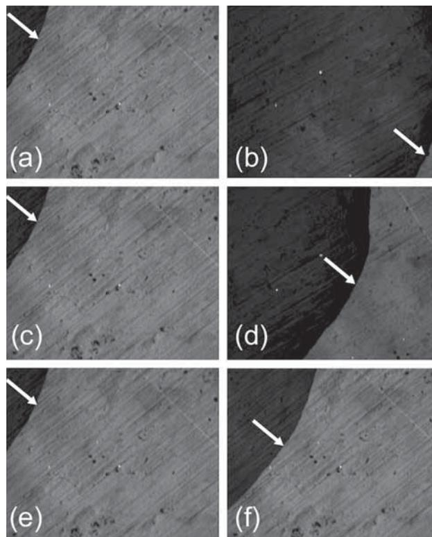
**Figure 2.** Images of the liquid front propagation on the gold-coated NAA for methanol, ethanol and isopropanol microdroplets. The arrows in (a), (c) and (e) mark the liquid fronts at  $t = 0$  s and the arrows in (b), (d) and (f) mark the liquid fronts at  $t = 5$  s.
