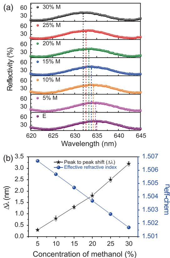
**Figure 4.** (a) Shifts in the peak reflectivity of the FP resonances for methanol–ethanol mixture with differing methanol content. The concentration of methanol is increased in steps of 5% and (b) variation in the effective refractive index of the mixture and FP mode shift with respect to the concentration of methanol in ethanol.
