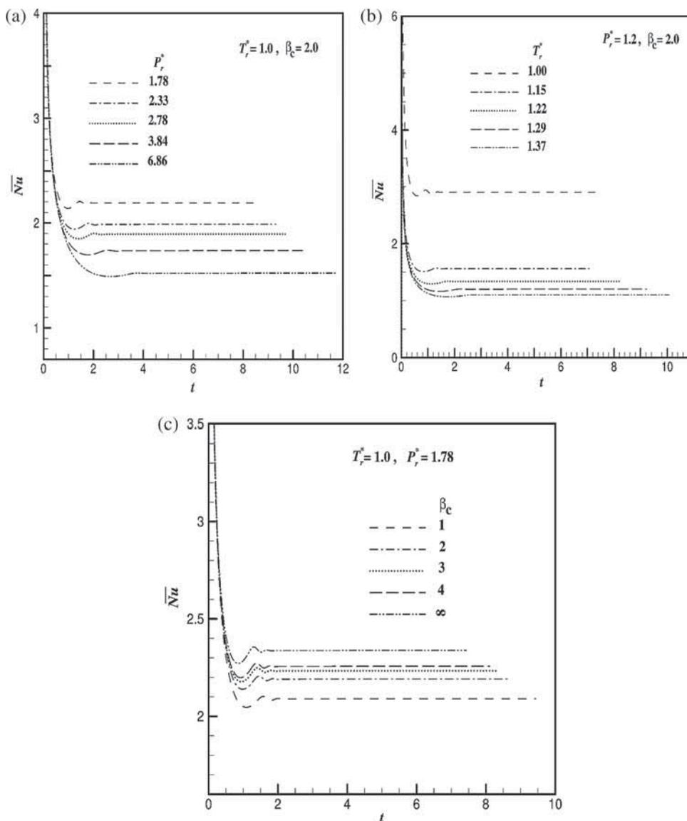
**Figure 13.** Average heat transport coefficient ( $\overline{Nu}$ ) for different values of (a)  $P_r^*$ , (b)  $T_r^*$  and (c)  $\beta_c$ .
