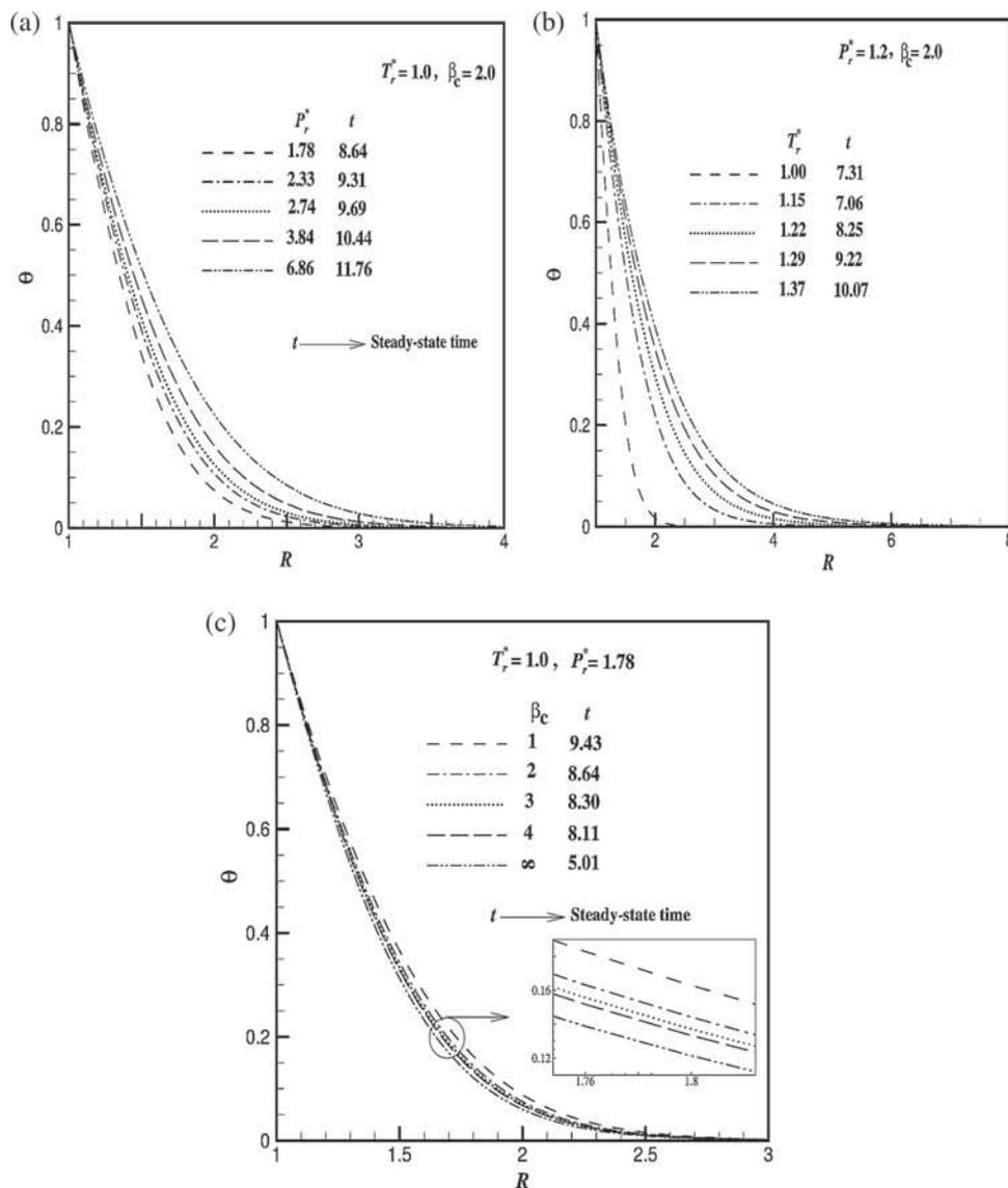
**Figure 11.** Time-independent state temperature profile ( $\theta$ ) against  $R$  when  $X = 1.0$  for different values of (a)  $P_r^*$ , (b)  $T_r^*$  and (c)  $\beta_c$ .
