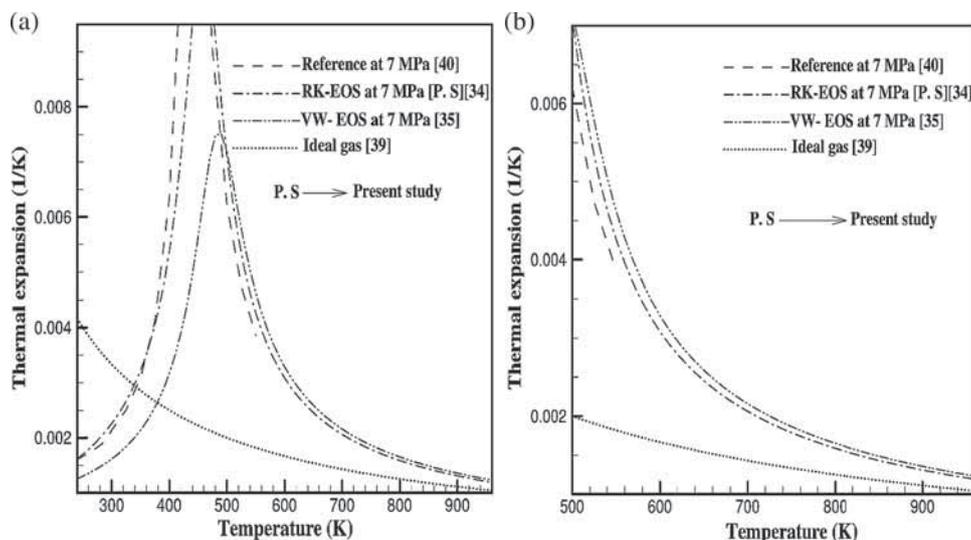
**Figure 3.** (a) Comparison of volumetric coefficient of thermal expansion ( $\beta$ ) of isobutane based on VW-EOS [35], perfect-gas assumption [39] and RK-EOS [34] with reference values [40] at 7 MPa and (b) an identical graph in the temperature range between 500 and 960 K.
