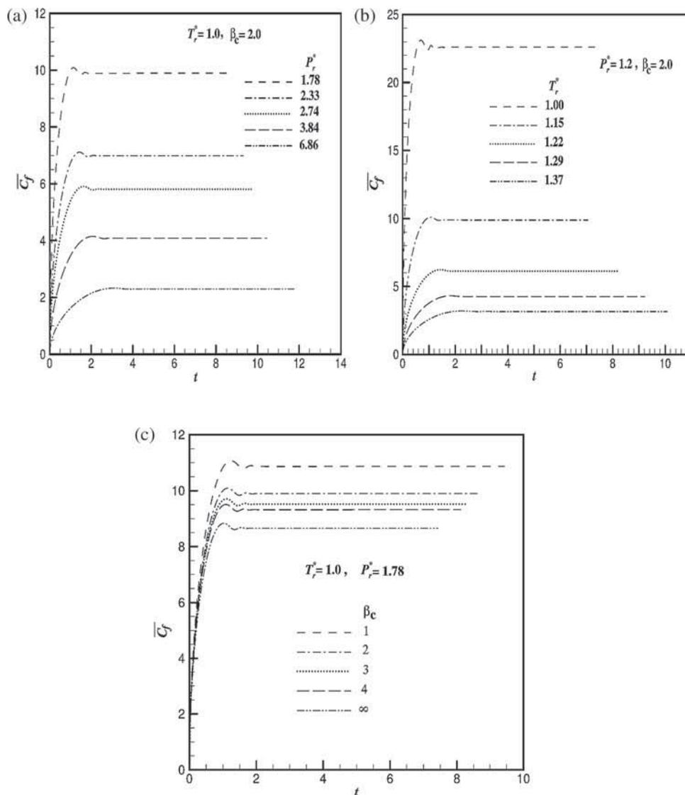
**Figure 12.** Average skin-friction coefficient ( $\bar{C}_f$ ) for different values of (a)  $P_r^*$ , (b)  $T_r^*$  and (c)  $\beta_c$ .
