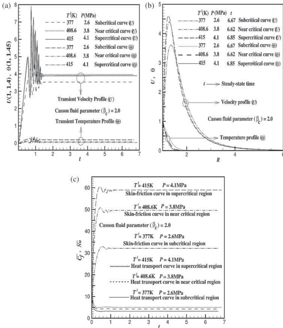
**Figure 14.** The curves in three regions for various pressures, temperatures and for fixed supercritical Casson fluid parameter,  $\beta_c = 2.0$ : (a) transient flow variables, (b) steady-state flow variables and (c) average skin-friction and heat transport coefficients.
