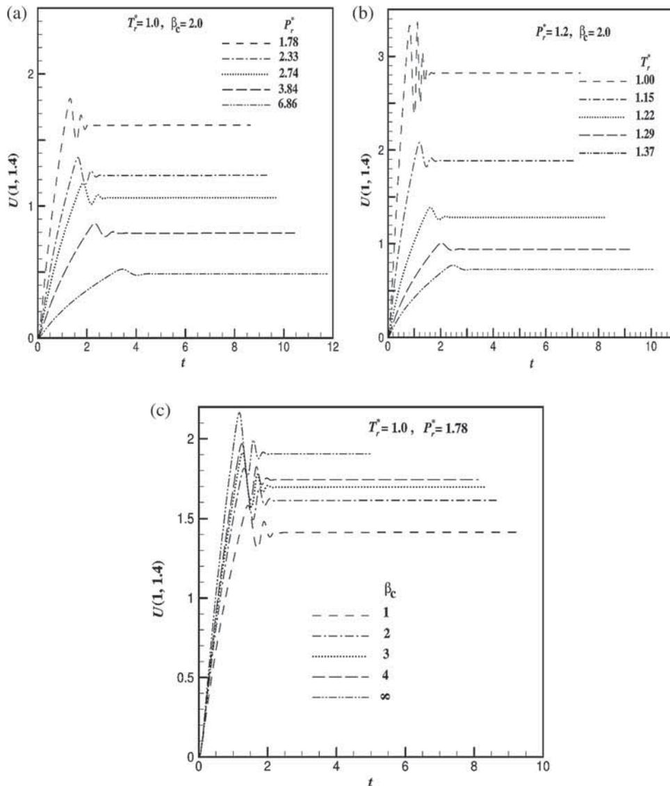
**Figure 7.** Numerically simulated velocity profile ( $U$ ) at (1, 1.4) against time ( $t$ ) for different values of (a)  $P_r^*$ , (b)  $T_r^*$  and (c)  $\beta_c$ .
