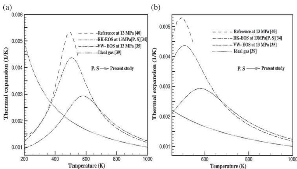
**Figure 4.** (a) Comparison of volumetric coefficient of thermal expansion ( $\beta$ ) of isobutane based on VW-EOS [35], perfect-gas assumption [39] and RK-EOS [34] with reference values [40] at 13 MPa and (b) an identical graph in the temperature range between 525 and 1000 K.
