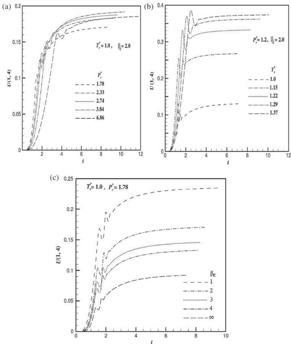
**Figure 8.** Numerically simulated velocity profile ( $U$ ) at (1, 4) against time ( $t$ ) for different values of (a)  $P_r^*$ , (b)  $T_r^*$  and (c)  $\beta_c$ .
