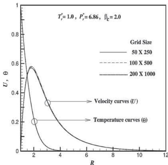
**Figure 2.** Grid independency test for the selection of grid size in the supercritical Casson fluid region.
