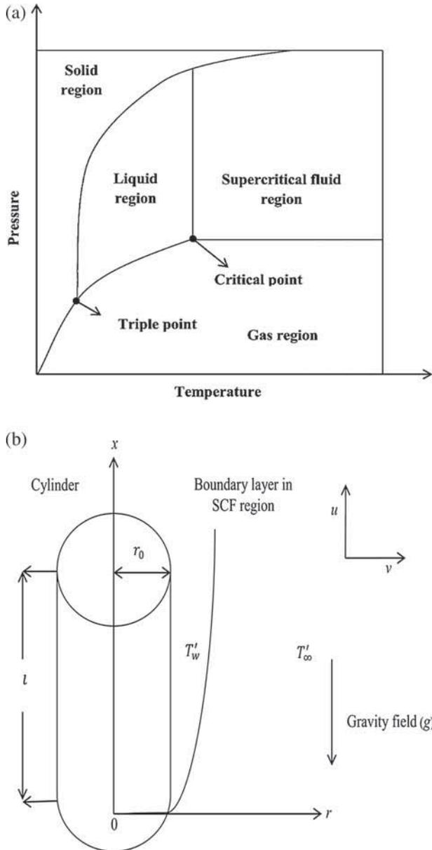
**Figure 1.** (a) Phase diagram and (b) physical model of the current problem.
