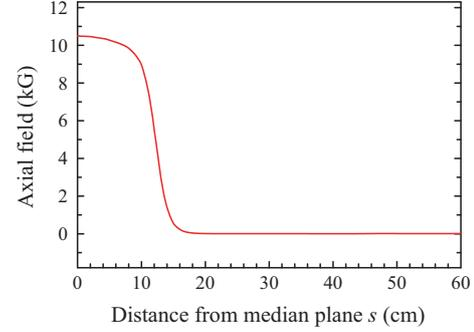
**Figure 2.** Variation of the magnetic field with distance  $s$  from the median plane along the cyclotron axis for 1056 A main magnet current. Data are obtained from 3D code.
