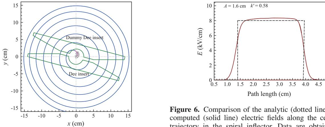
**Figure 5.** The projection of the inflector, location of the accelerating gaps in the central region and accelerated orbits of  $O^{6+}$  ions from 38.45 keV to 3 MeV. The pink solid line indicates the projection of the central ion trajectory of the inflector in the median plane.
