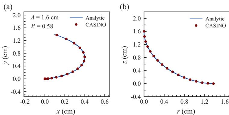
**Figure 3.** Central orbit for an analytic electric field distribution: (a)  $x$ - $y$  projection and (b)  $r$ - $z$  projection. The solid line and the filled circle represent the results obtained from analytical calculations and CASINO, respectively.
