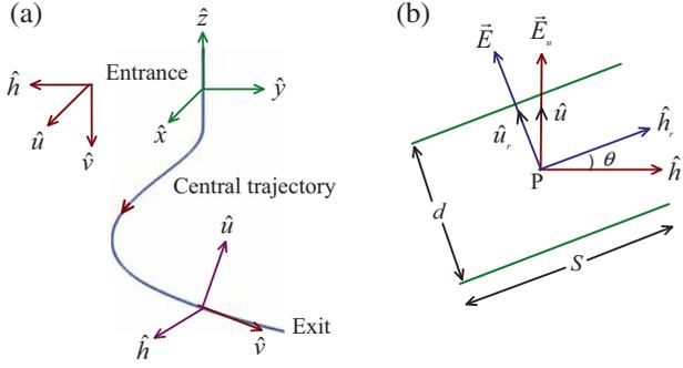
**Figure 1.** A schematic of (a) fixed right-handed Cartesian ( $x, y, z$ ) with basis vectors  $\hat{x}, \hat{y}$  and  $\hat{z}$  and an optical ( $u, h, v$ ) coordinate system with basis vectors  $\hat{u}, \hat{h}$  and  $\hat{v}$  and (b) spiral inflector geometry as viewed from a plane perpendicular to the central trajectory. Here  $d$  is the electrode spacing and  $S$  is the width of the electrodes.
