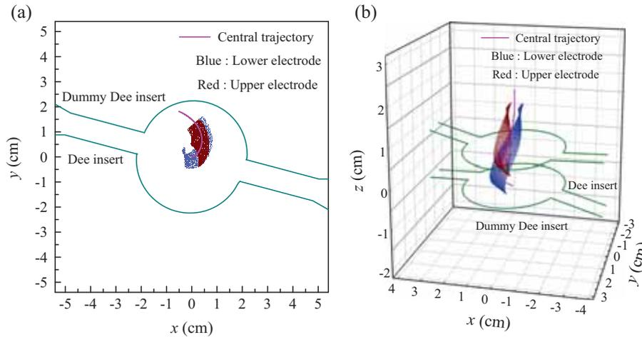
**Figure 4.** Schematic shape of the spiral inflector: (a) the  $x$ – $y$  projection of the two-electrode shape and (b) biased electrode geometry. The central ion trajectory, Dee and Dummy Dee inserts are also shown in the plot.
