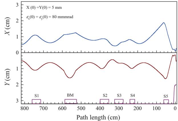
**Figure 10.** Optimised beam envelopes along the  $x$  and  $y$  directions for the input beam with  $X(0) = Y(0) = 5$  mm,  $P_x(0) = P_y(0) = 0$  mrad and equal emittance  $\varepsilon_x(0) = \varepsilon_y(0) = 80$  mm mrad. The relation between the Cartesian  $(x, y, z)$  and optical  $(u, h, v)$  coordinated system in the spiral inflector is explained in figure 1.
