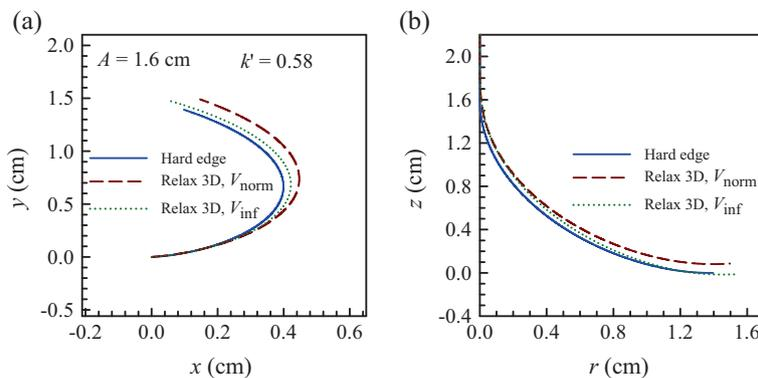
**Figure 7.** Comparison of the central orbit obtained from the hard edge electric field (solid line), a field from RELAX3D (dashed line) with  $V_{\text{norm}}$ , and a field from RELAX3D with a reduced voltage  $V_{\text{inf}}$  (dotted line): (a)  $x$ - $y$  projection and (b)  $r$ - $z$  projection.
