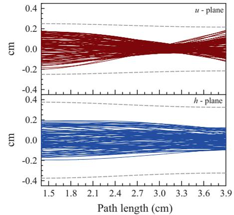
**Figure 9.** Paraxial ion trajectories through the spiral inflector in both the  $u$  and  $h$  planes for the RELAX3D electric field with reduced potential  $V_{inf}$ . Dashed lines represent the available electrode aperture.
