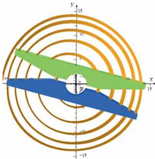
**Figure 12.** Trajectories of 500 particles for the first few turns in the central region with an optimised input condition at the matching point. Dee and Dummy Dee inserts are also shown. To make the trajectory visible, Dee ( $180^\circ$ ) and Dummy Dee are not plotted.
