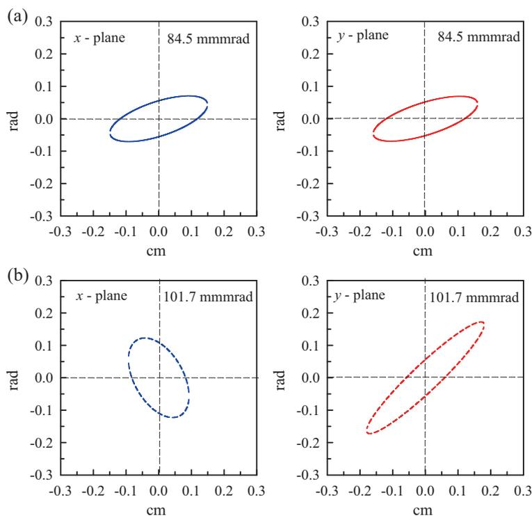
**Figure 11.** The phase ellipses at the (a) inflector electrode entrance and (b) matching point for the optimised values of the injection line parameters. The matching point is at  $x = -0.39$  cm and  $y = 1.75$  cm in the median plane.
