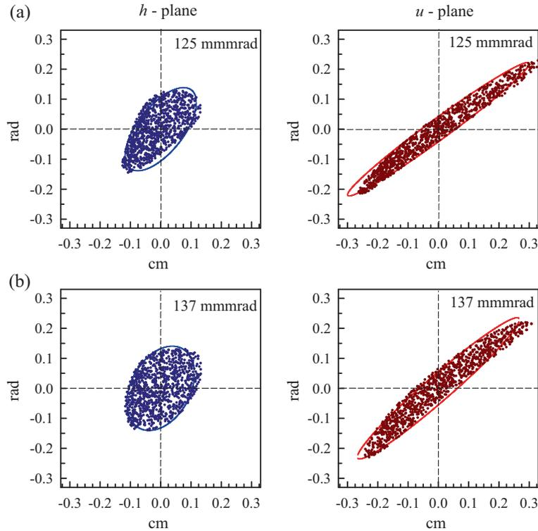
**Figure 8.** Phase-space ellipses in the  $h$  plane and  $u$  plane at the inflector effective exit: **(a)** represents the phase ellipses for a hard edge electric field and **(b)** represents the phase ellipses for RELAX3D field with reduced potential. Input beam parameters are  $U(0) = H(0) = 2$  mm,  $P_u(0) = P_h(0) = 0$  mrad and  $\varepsilon_u(0) = \varepsilon_h(0) = 80$  mm mrad for both the cases at  $s_0$ .
